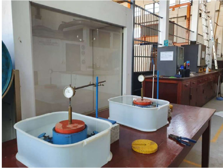
Plate 3-7: Specimen soaking and preparation for CBR test
