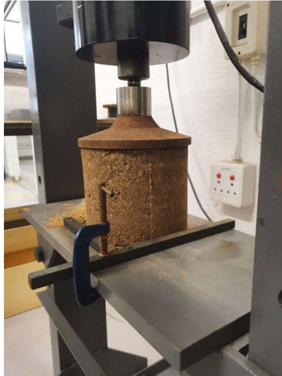
Plate 3-9: UCS Test Setup
