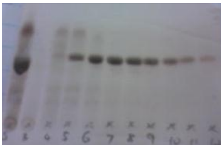
Figure 2.2: TLC plate showing fractions collected from a reverse phase chromatography column in the manifold assembly.
