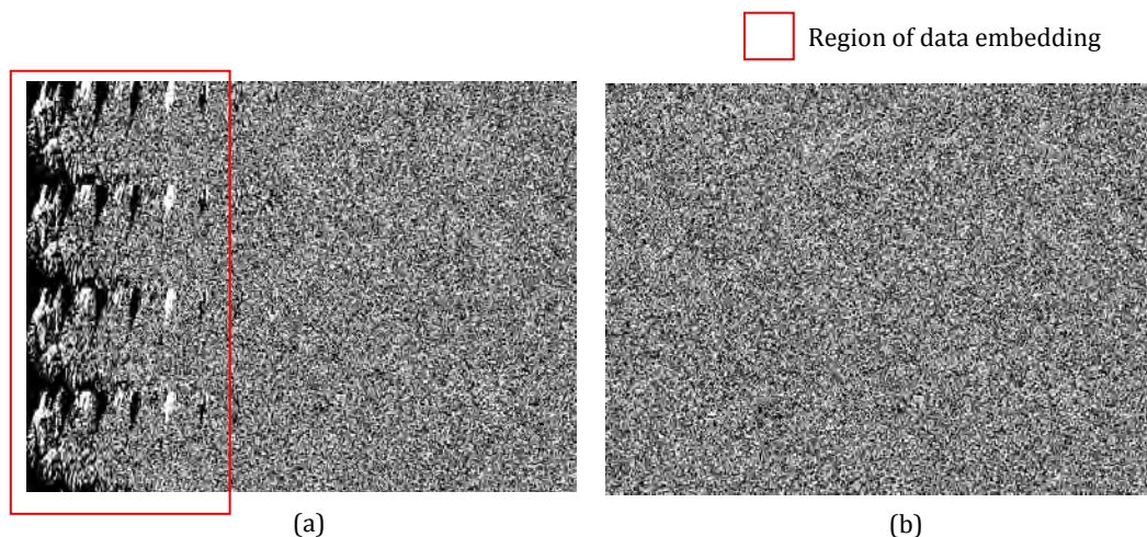
Figure 2-7. LSB plane of stego-image (a) and original cover image (b)
