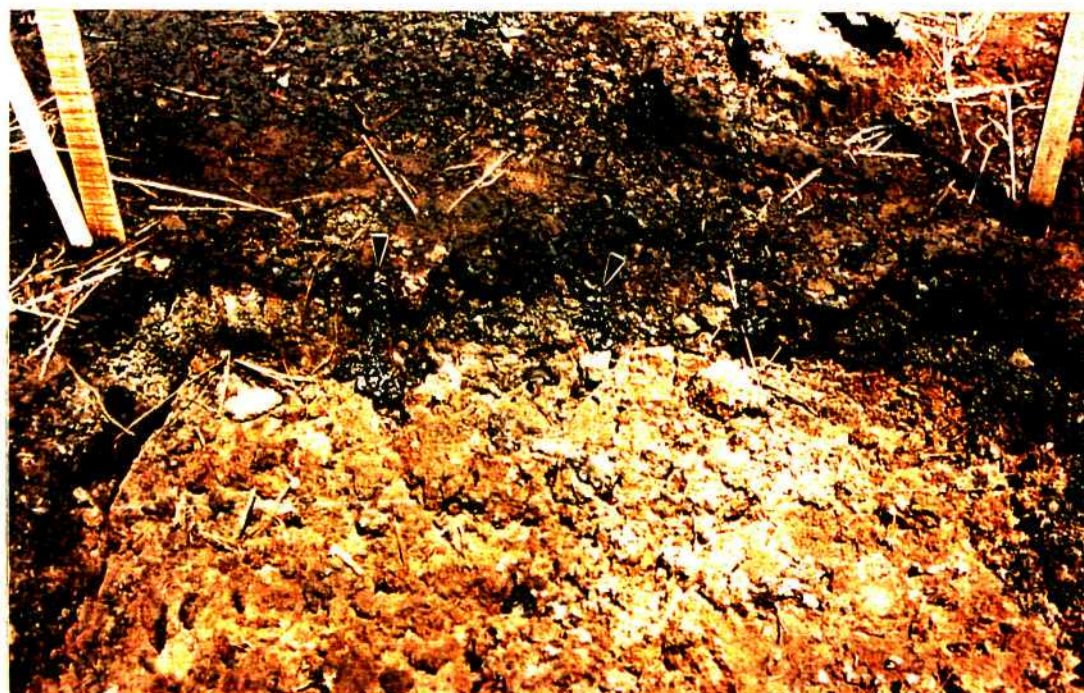
Plate 1b: Close-up of a soil sampling plot with free-product contamination indicated.
