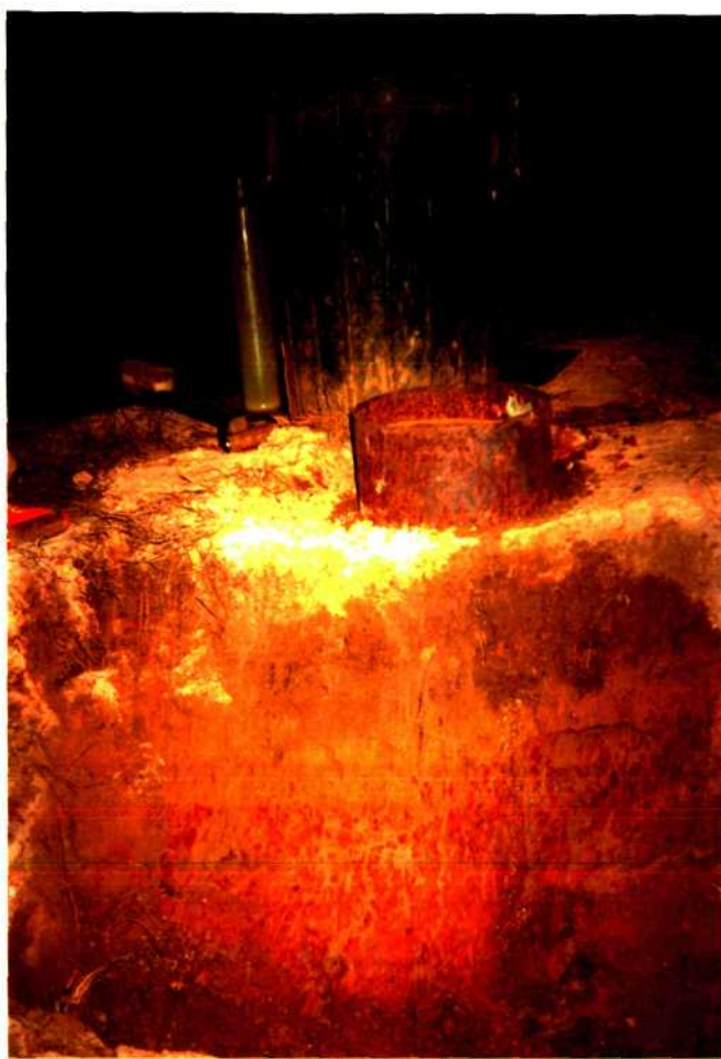
Figure 61. Preferential flow pathways illuminated with a fluorescent dye at Pit 3.
