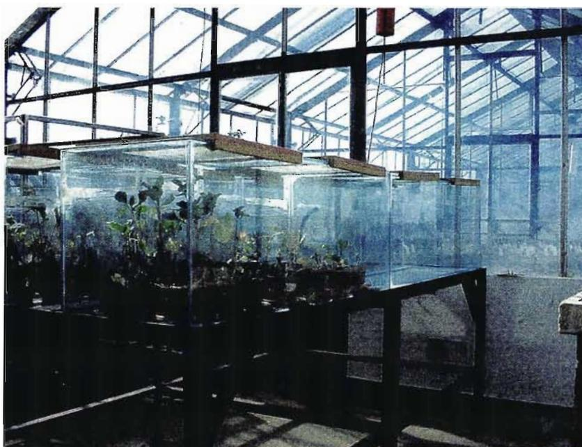
Figure 2.4 Glass tanks used as rearing chambers in the glasshouse under wet wall cooling.
