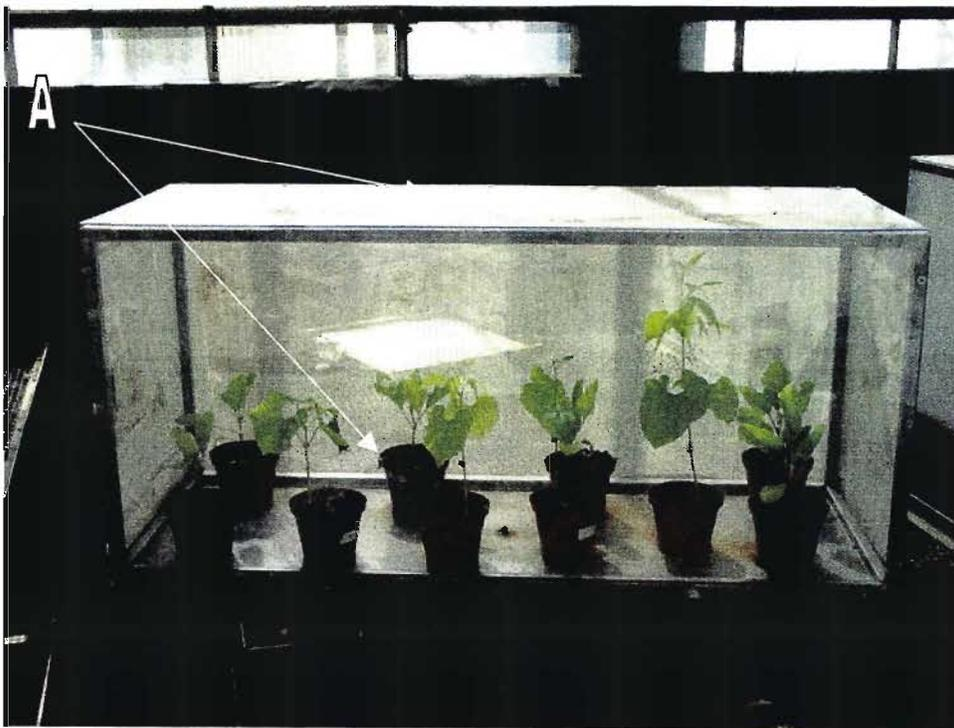
Figure 2.6 Ventilated rearing chambers. A: Perspex covering for the lid and front. The rest of the cage is covered with insect netting for ventilation.
