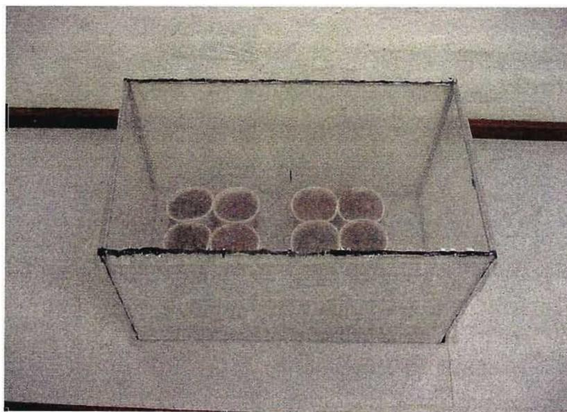
Figure 2.2 Insect rearing chamber used to rear aphids and whiteflies under laboratory conditions.
