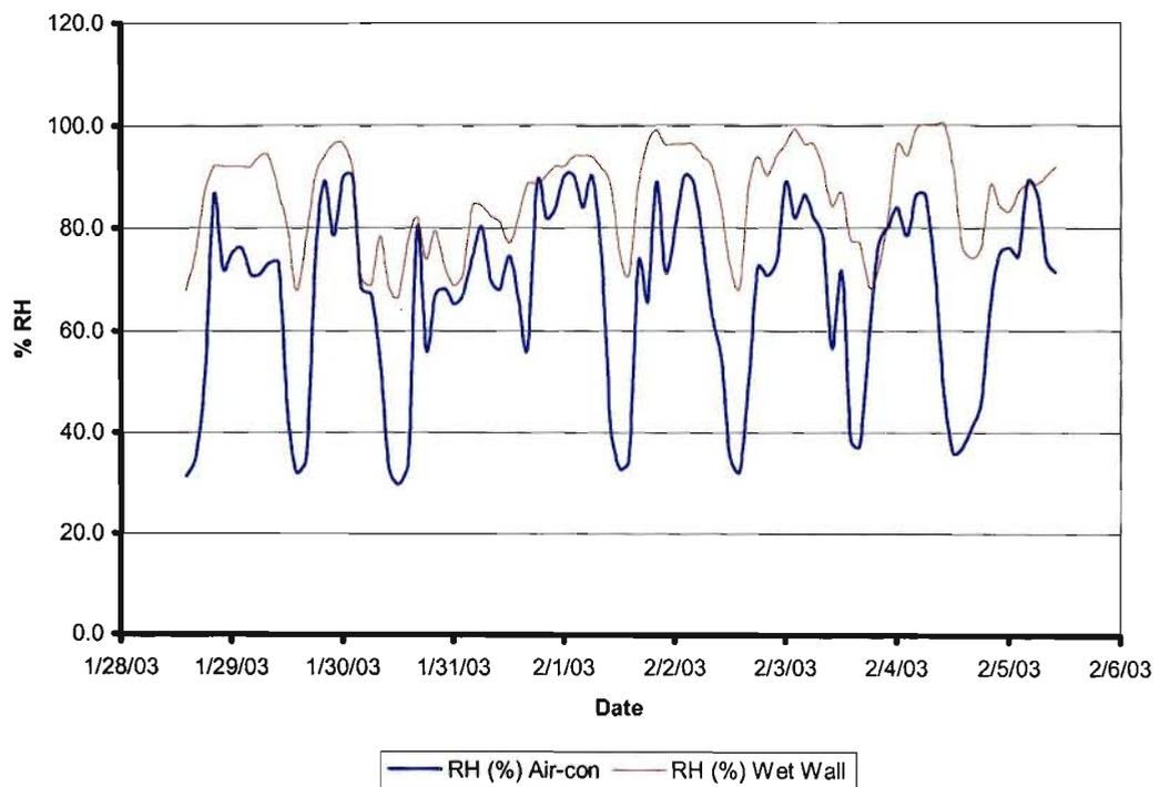
Figure 2.7 Temperature (top) and relative humidity (bottom) differences between the industrial air-conditioning system and the wet wall cooling system measured over a 9d period.
