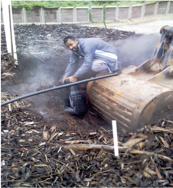
Plate 4.16: Sampling of the DAT Window using an excavator
