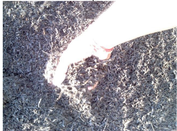
Plate 5.4: Particle sizes of 10mm to dust
