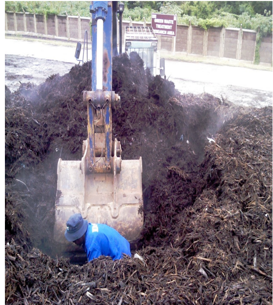
Plate 4.17: Sampling of the TTW using an excavator
