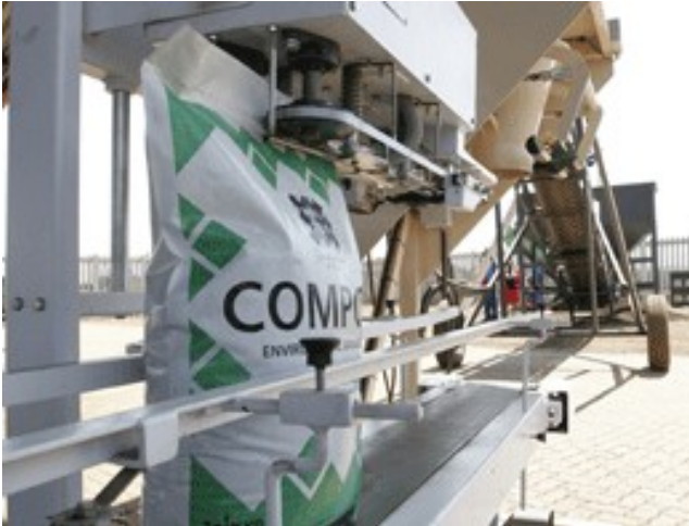
Plate 2.9: Bagging Machine of Compost Final Product
