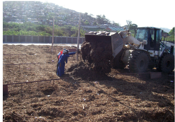
Plate 4.8: Placement of wetted garden refuse by FEL in windrow
