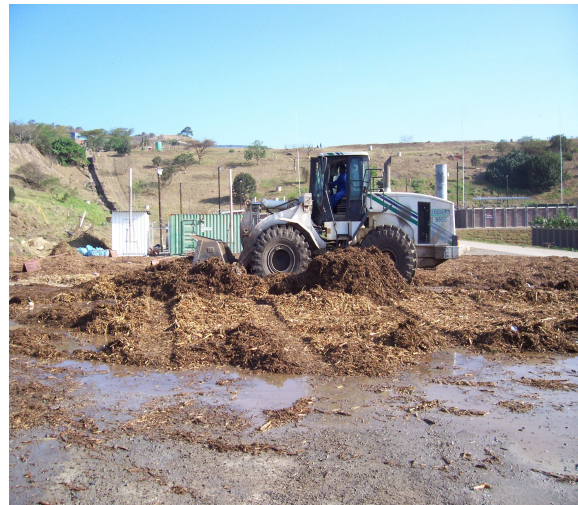
Plate 4.6: FEL mixing and homogenizing water into shredded material
