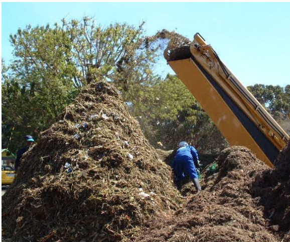
Plate 2.3: Manual Sorting of contamination
