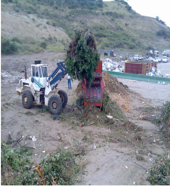
Plate 3.8: Front end loader feeding the shredder with mixed garden refuse
