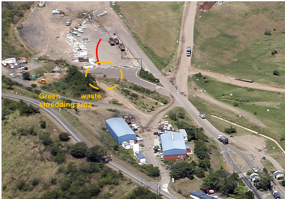
Figure 3.7: Flow path of garden refuse for shredding on transfer station
