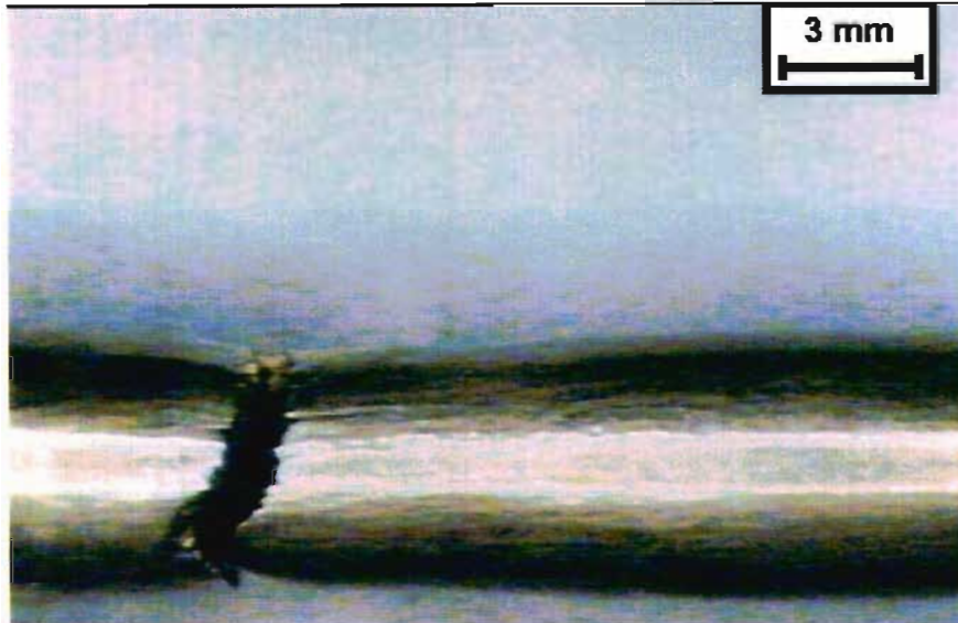
Figure 2.6 Broken out of gauge length 75% warm rolled sample A1 as reported on the test certificate
