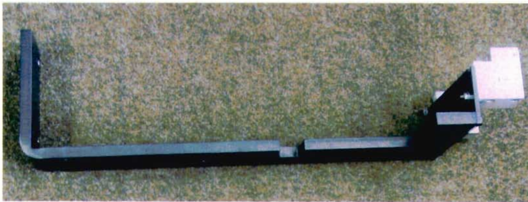
Figure 2.15 Rigid test - rig which allows keeping the meter at a permanent position during all tests
