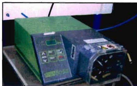
Figure 10.3: Photograph of the Watson Marlow Peristaltic Pump
