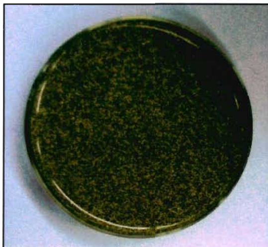
Figure 10.1: Photograph of a handful of TP 207 resin in the Hydrogen form
