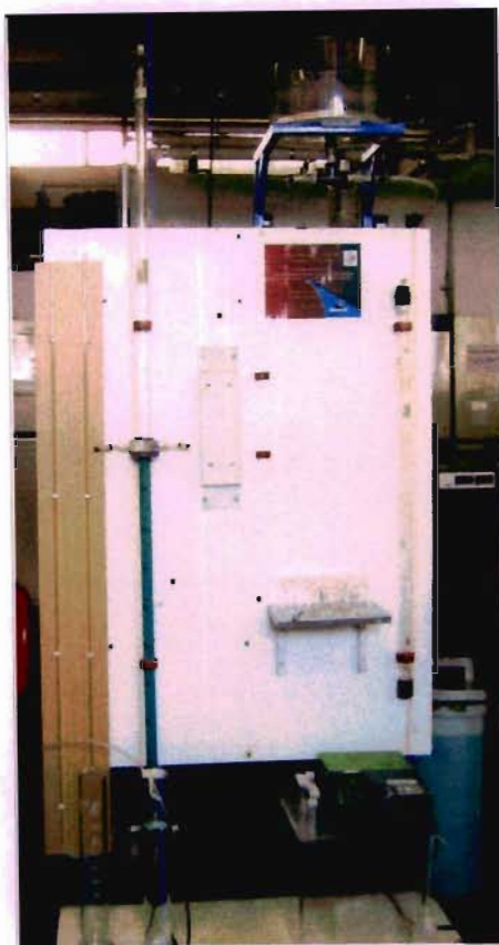
Figure 10.9: Photograph of the Fluidized Bed at the End of Operation with resin fully loaded with Copper
