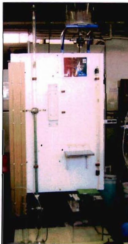
Figure 10.8: Photograph of the Fluidized Bed during Operation with Copper loading onto the resin
