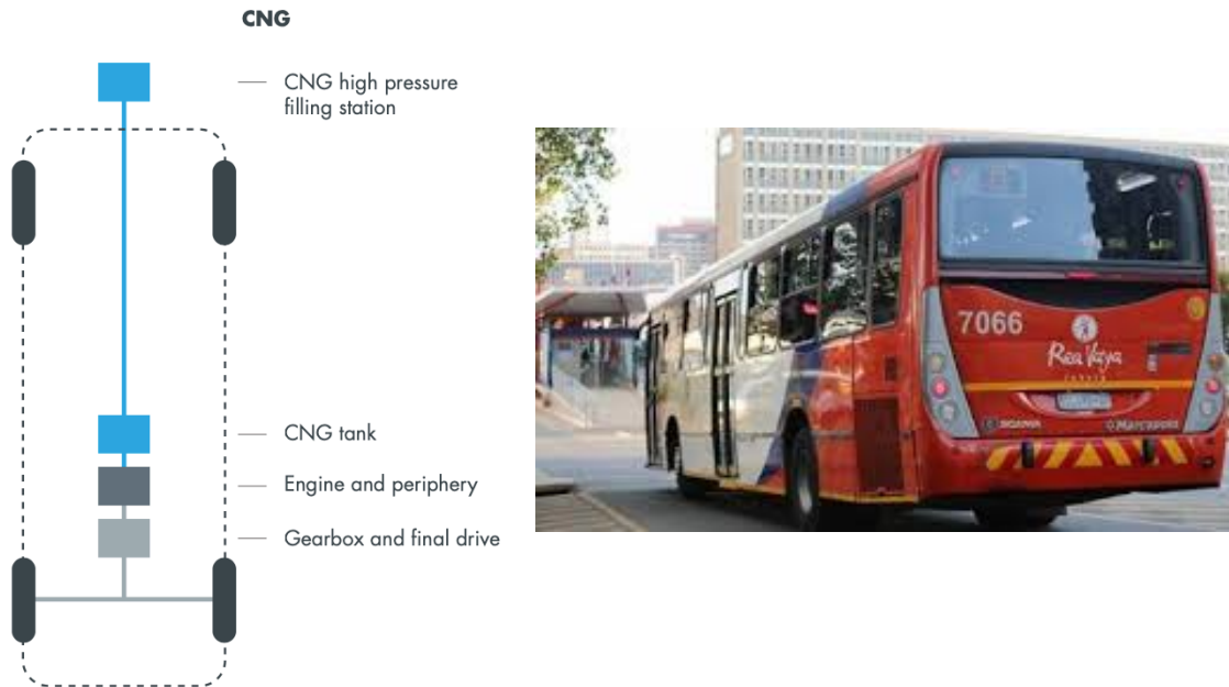
Figure 14 Showing: Euro VI CNG bus powertrain layout (left) (CIVITAS, 2016) and CNG Rea Vaya Bus Johannesburg (right) (Rea Vaya, 2020)
