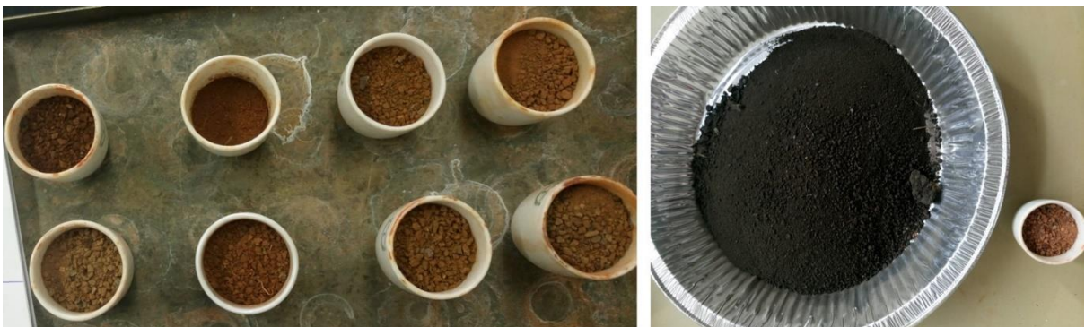
Figure 4.6: Crucibles with soil after undergoing loss on ignition and a comparison of the soil sample before and after undergoing loss on ignition
