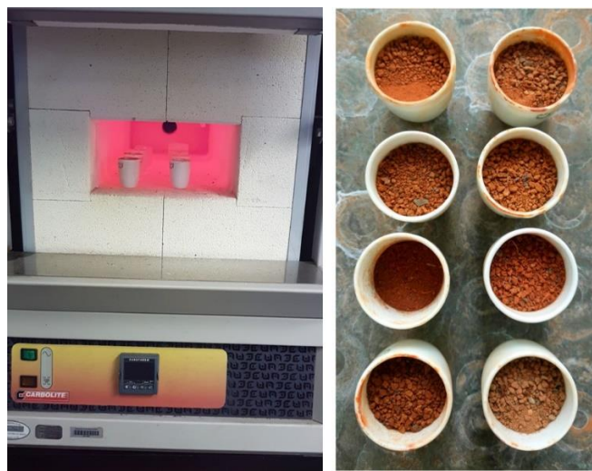
Figure 4.8: Sediment samples immediately after sequential loss on ignition
