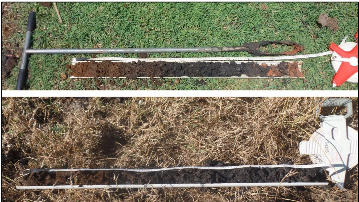
Figure 4.2: Examples of sediment cores extracted with the soil auger
