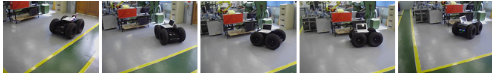
FIGURE 5.28: Screenshots from video of the RMP400 turning in a tight space
