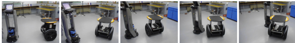
FIGURE 5.26: Screenshots from video of the RMP200 obstacle avoidance
