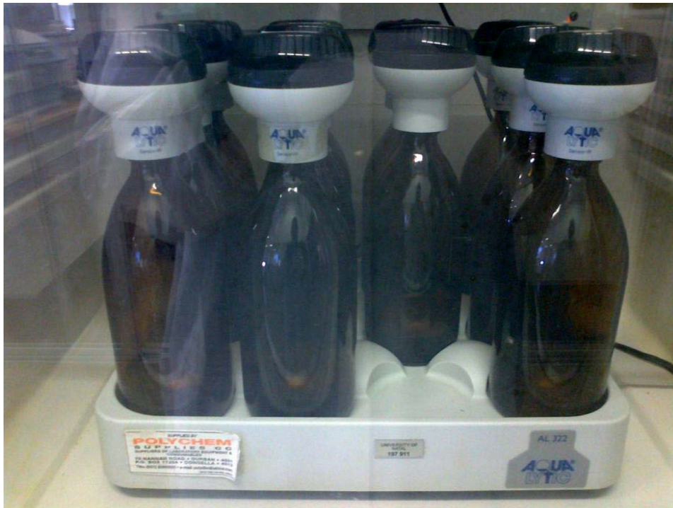
Figure 3-27 BOD test in progress
