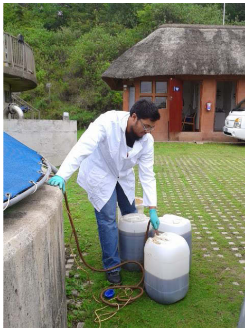
Figure 3-4 Sampling of treated leachate in progress
