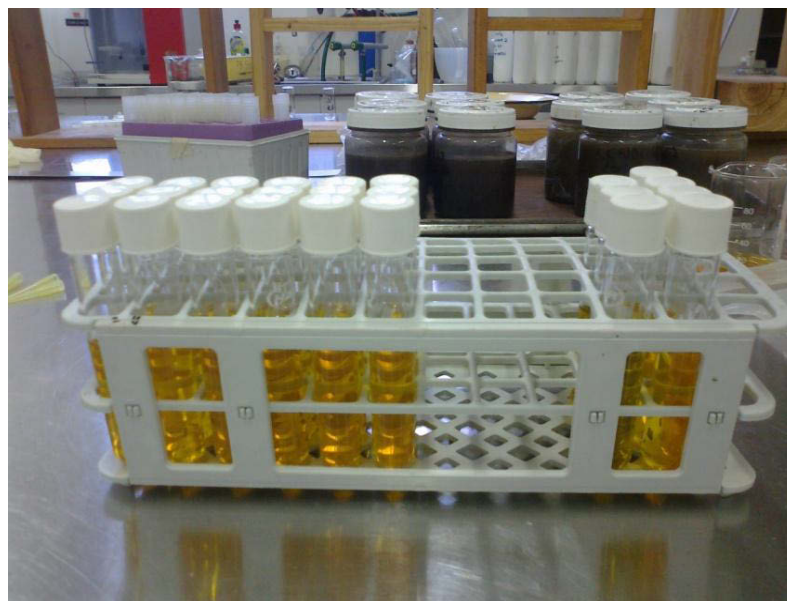
Figure 3-25 COD test tubes
