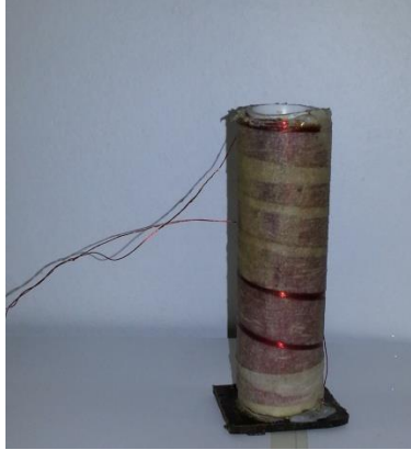
Figure 5. 5 Picture of the primary coil built.
