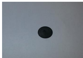
Figure 6. 2 Top view of YBCO disc sintered in the tube furnace.
