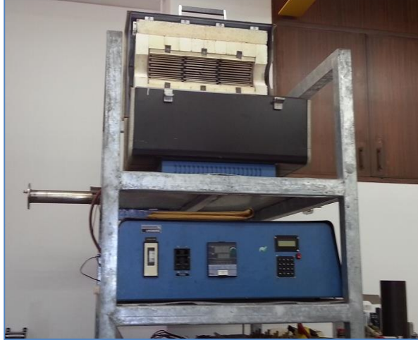
Figure 6. 1 Tube furnace used for the sintering of YBCO pellets.
