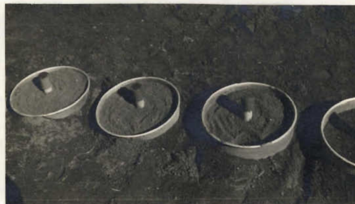
1b Filled pots showing probe tubes
