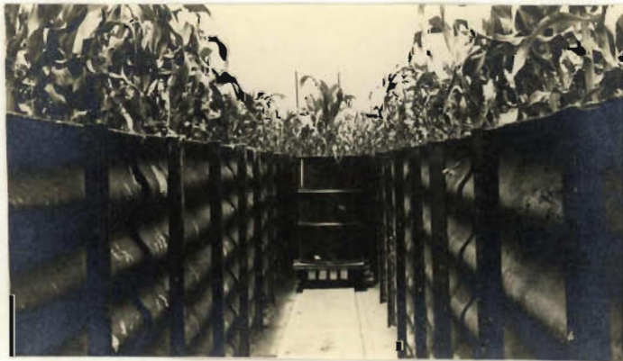
2b Lysimeters on trucks in trench
