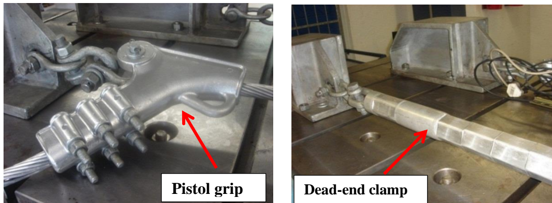
Figure 3-7 Photo of pistol grip; Pelican (left) and dead-end clamp: Bersfort (right)
