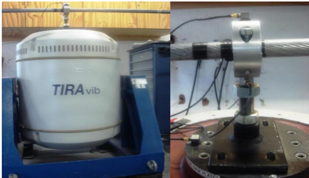
Figure 3-2 Electrodynamic vibration exciter: shaker (left) and rigid connection (right)
