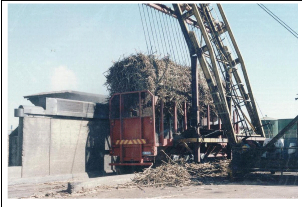
Figure 2.11 An example of a spiller offloading a load of cane onto the spiller table (Simpson, 2004).
