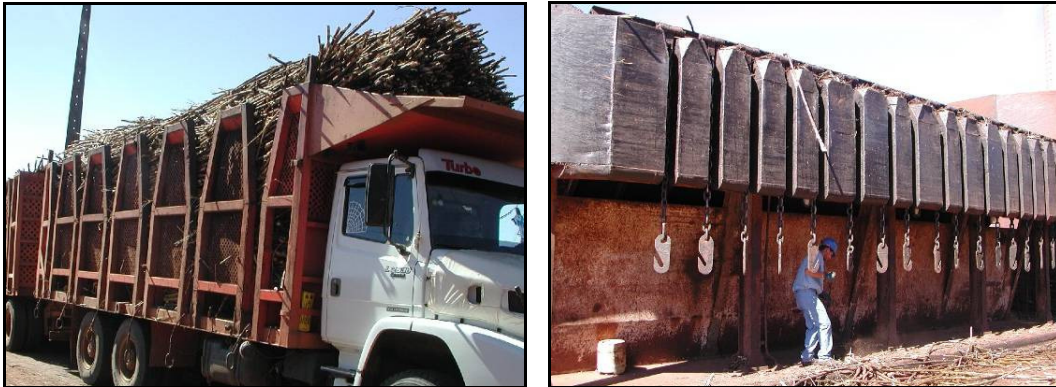
Figure 7.3 A typical Brazilian sugarcane vehicle (left) showing the spaces provided for feeding the offloading cables with the cables inserted ready for offloading, together with the spiller mechanism (right) to which the cables are temporarily attached to offload the sugarcane.
