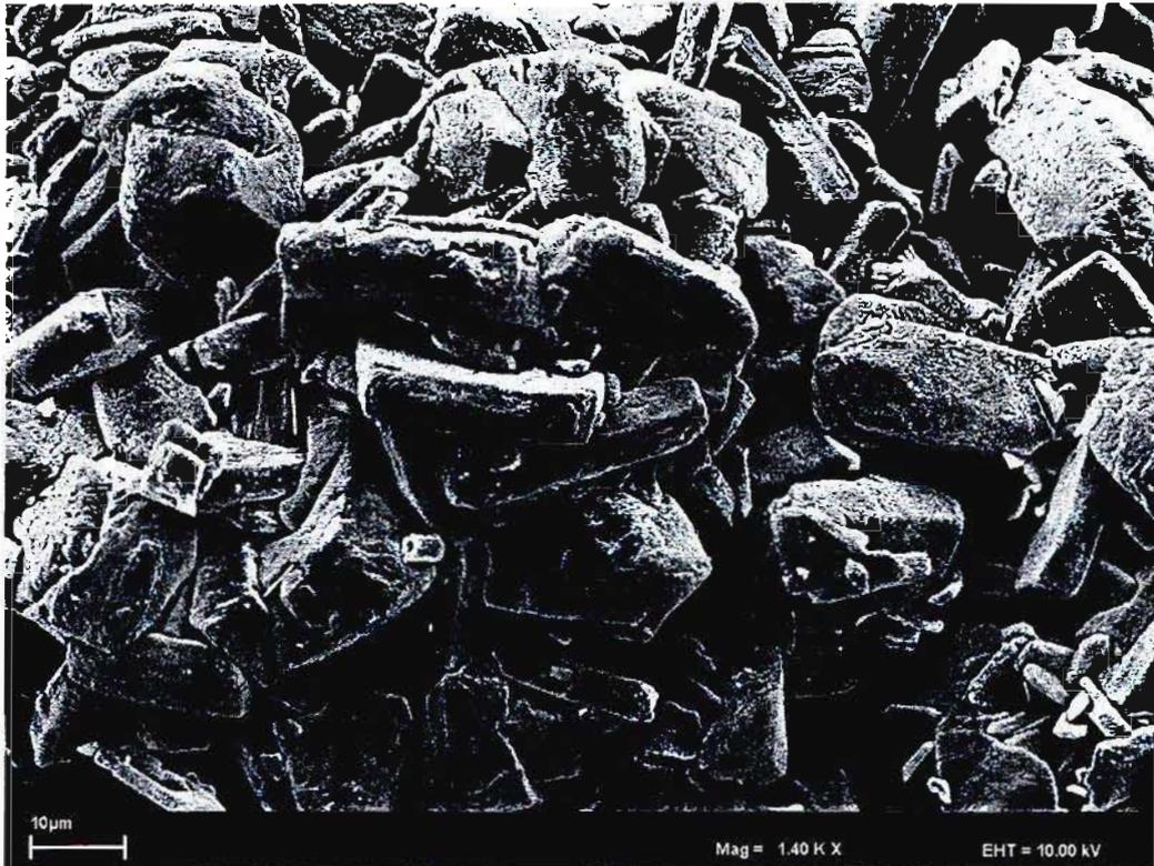
Figure 3AL: SEM Image of V<sub>2</sub>O<sub>5</sub>
