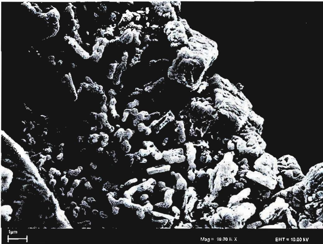
Figure 3AN: SEM Image of V<sub>2</sub>O<sub>5</sub>
