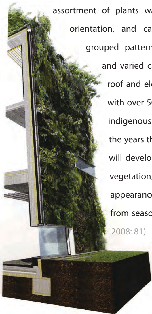
FIG 5.59: THREE DIMENSIONAL SECTION THROUGH THE FACADE OF THE FACILITY (LEER, 2008: 68).
