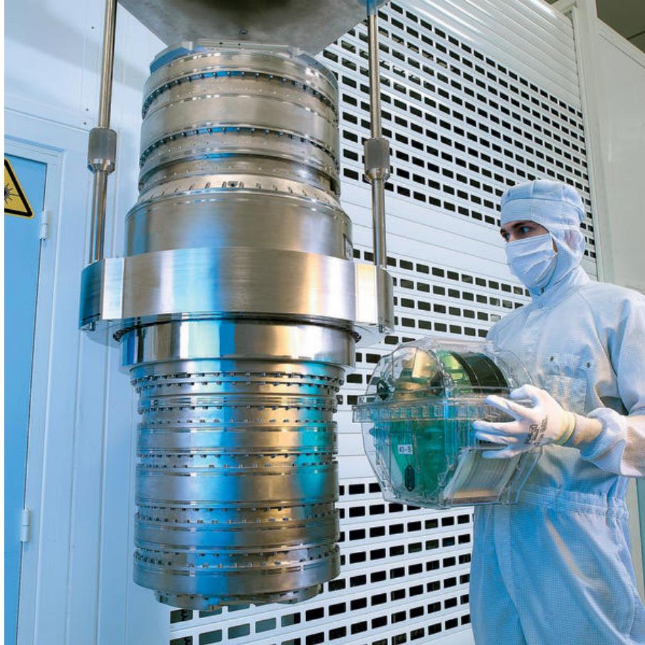
Figure 4.2: Zeiss® Starlith 1000 Lithography Lens Opto-Mechanical Assembly, Courtesy Electronics Production and Test [80]
