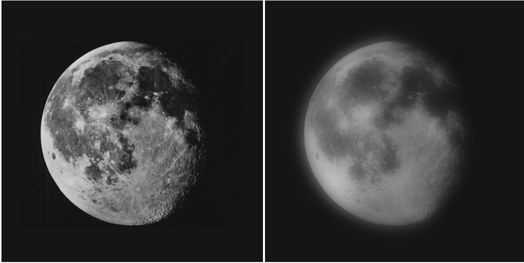
Figure 4.3: Moon Image with Low Stray Light (left) and Simulated Stray Light (right)
