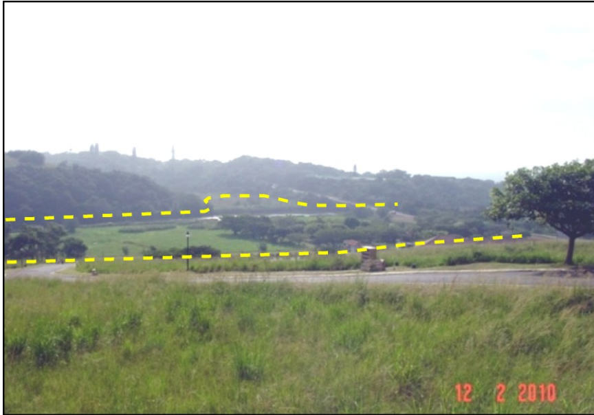
Figure 5.12. View of the Zotshe River floodplain at Site 2 (Fig. 5.11). The yellow dashed line marks the maximum flood elevation as defined by flood deposits.
