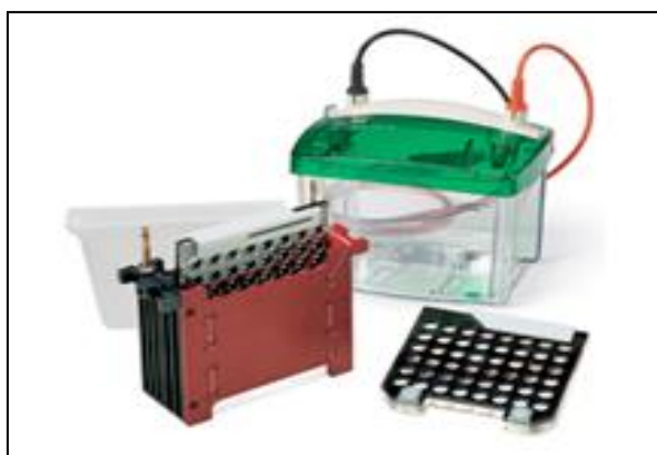
Figure 2.4. Equipment used for PAGE gel electrophoresis. The tank, gel holder cassette and electrode assembly are presented. Image adapted from www.bio-rad.com .
