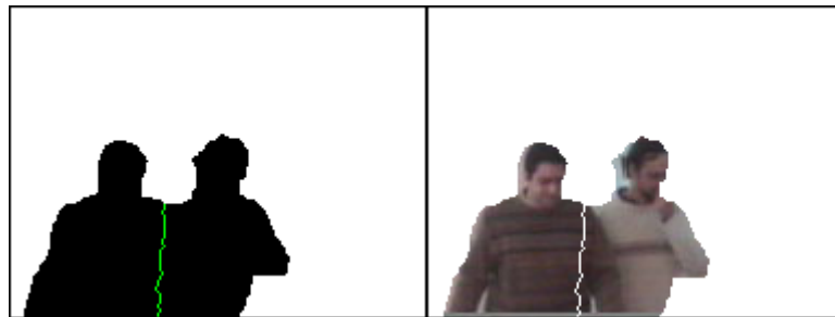
Figure 4.15: Results when using the greedy algorithm. Left: vertical seam calculated. Right: overlaid over original frame.
