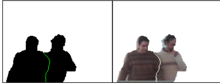
Figure 4.16: Results when using the dynamic programming algorithm. Left: vertical seam calculated. Right: overlaid over original frame.
