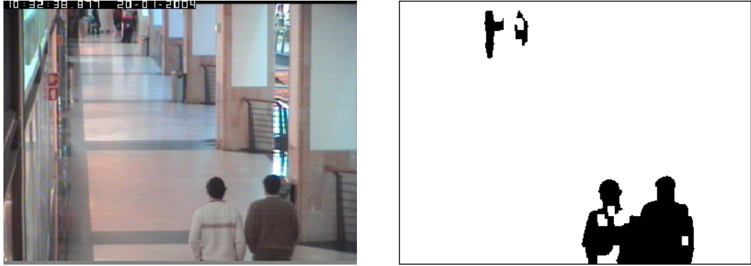
Figure 3.5: Results of the application of the mixture of Gaussians for background subtraction. The left image is the original image and the right one is extracted foreground regions.
