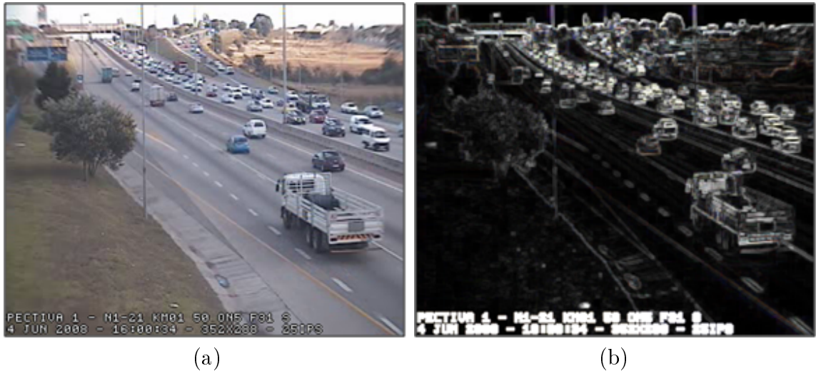
Figure 4.4: (a): Original image. (b): Edge detection by the external morphological gradient.
