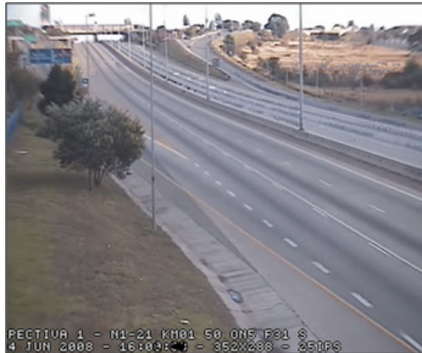
Figure 4.5: The background of the traffic scene is calculated using a mixture of Gaussians. The edges calculated on this image are then removed from the original edge map, leaving only the vehicles.
