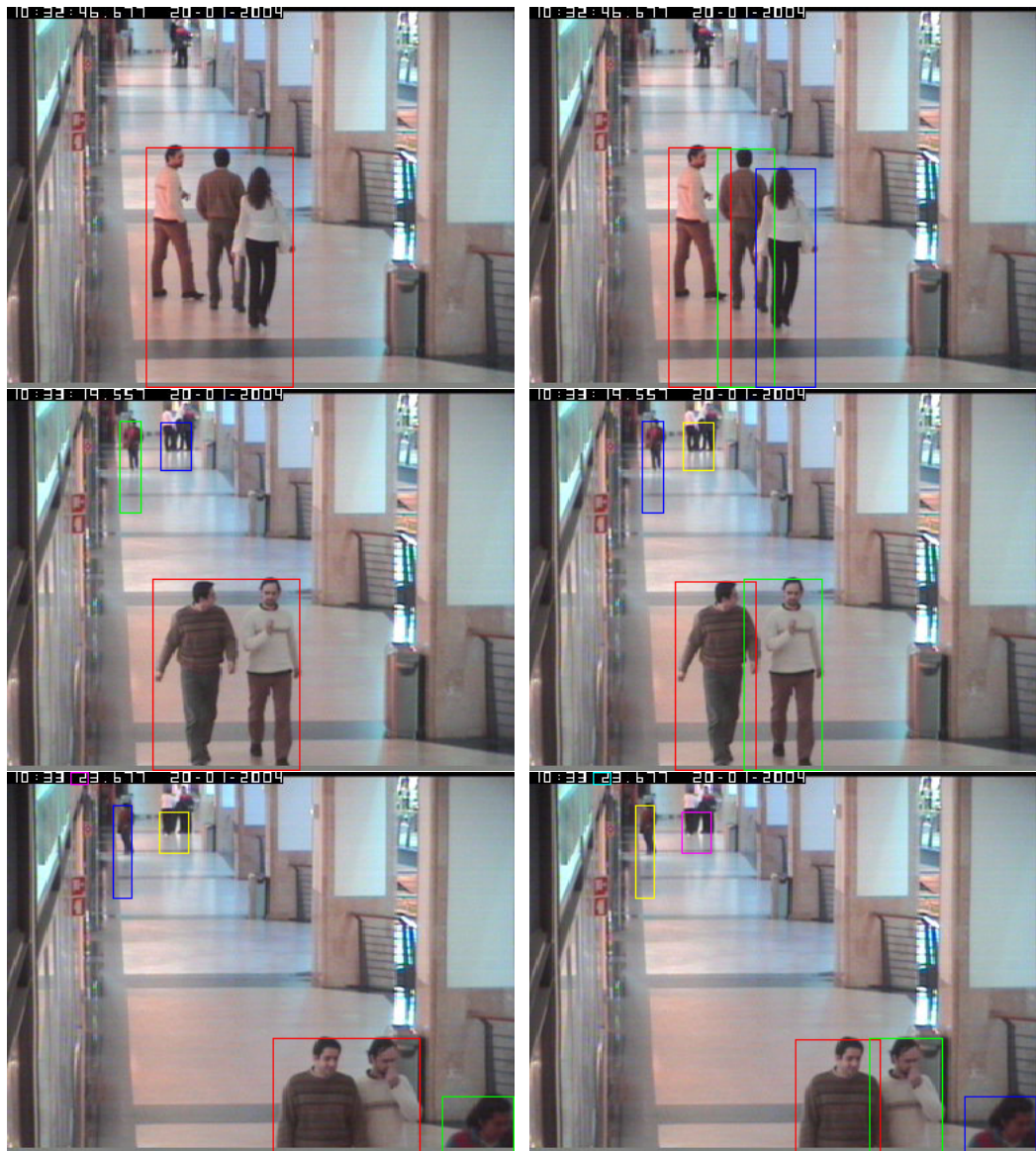
Figure A.3: Here is an example of the technique discussed in Chapter 4, section 4.2. On the left: a simple tracking algorithm is in place. And on each image's corresponding right-hand side one can see the results of same tracking algorithm with just the structural analysis technique in place. Notice how the objects are uniquely tracked on the right-hand side when compared with the left-hand side.
