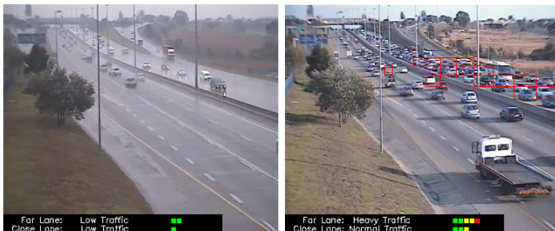
Figure 4.6: Two frames displaying the qualitative results for two scenes. The contextual description of the traffic status as well as a visual representation is shown in the image. Areas of congestion are highlighted on the actual frames. The scene on the left maintains a low traffic status on both carriageways. It also contains no areas of congestion. The scene on the right maintains a heavy traffic status on the far carriageway and a normal traffic status on the closer carriageway. Several areas of congestion are highlighted, especially in the far carriageway. (See Figure A.2 in the Appendix for additional results.)
