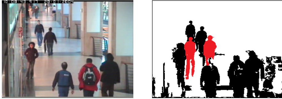
Figure 3.4: Example of the ghosting problem encountered when using selective updating. Left: original frame. Right: foreground mask with highlighted areas indicating ghosts
