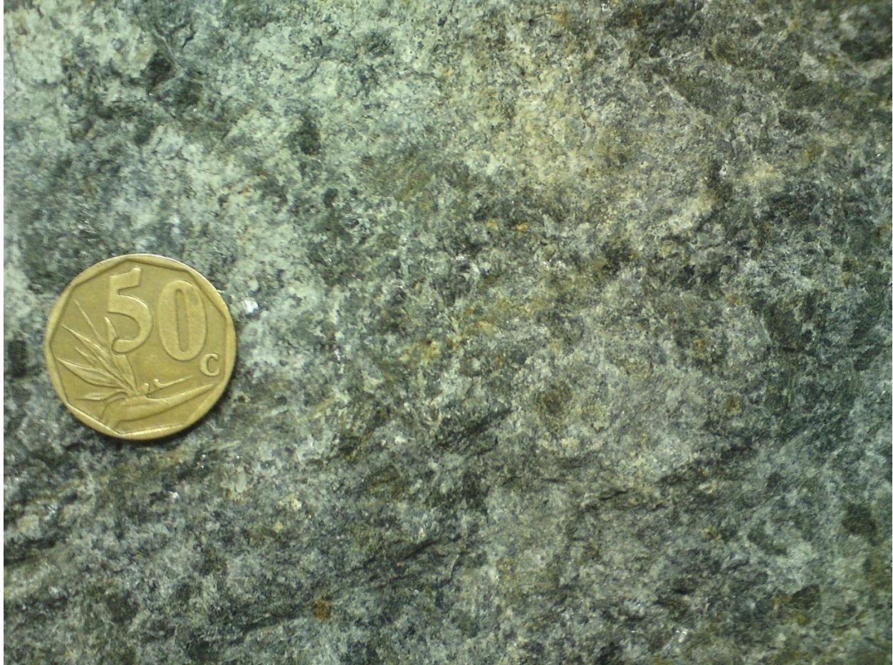
Plate 2.4 Weathered surface of medium-grained pyroxenite from the Mambulu Complex. Coin shown for scale, diameter of 22mm (photograph by I. Mustapha).
