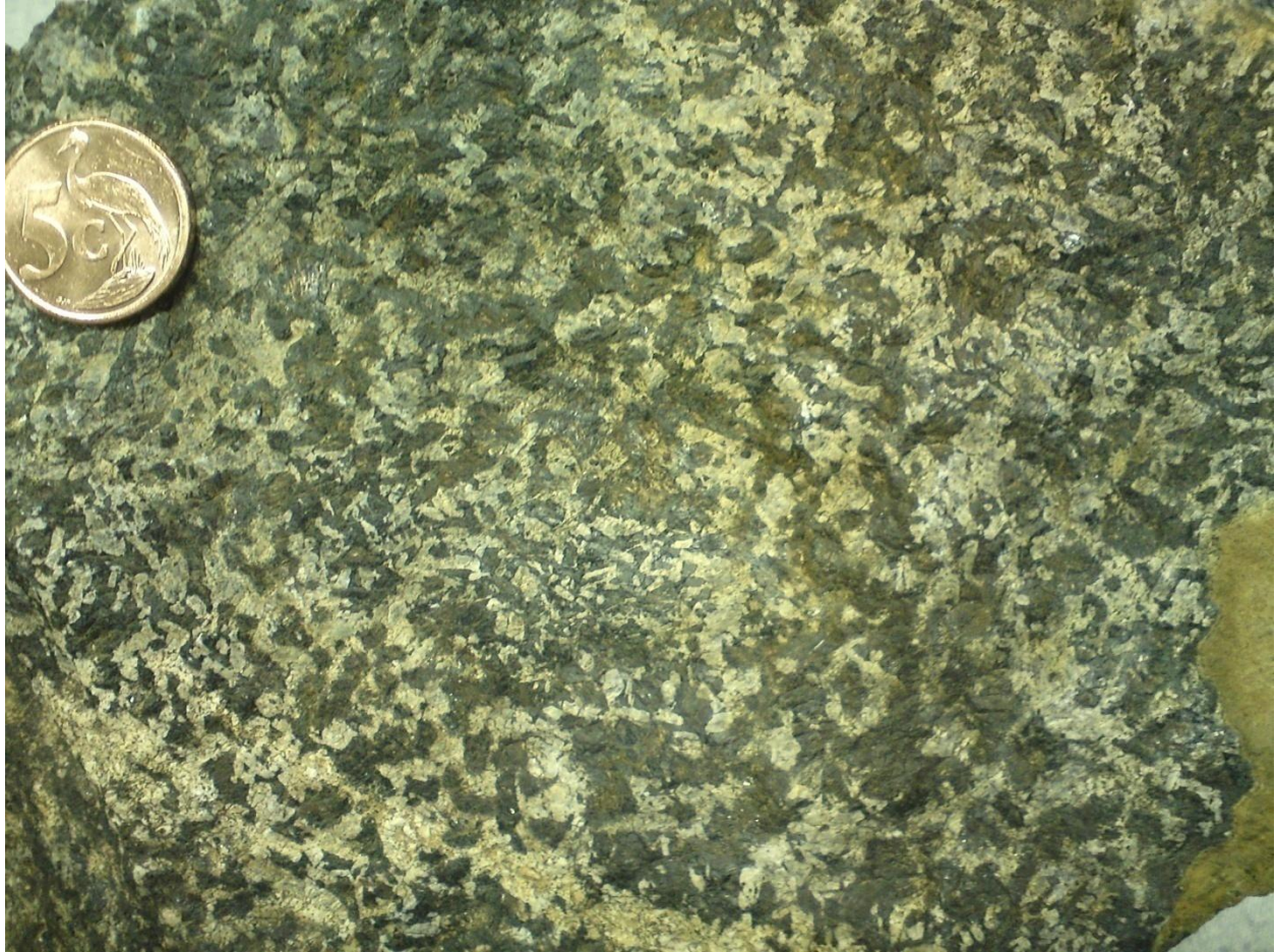
Plate 2.2 Weathered surface of coarse-grained leuco-gabbro from the Mambulu Complex. Coin shown for scale, diameter of 20mm (photograph by I. Mustapha).
