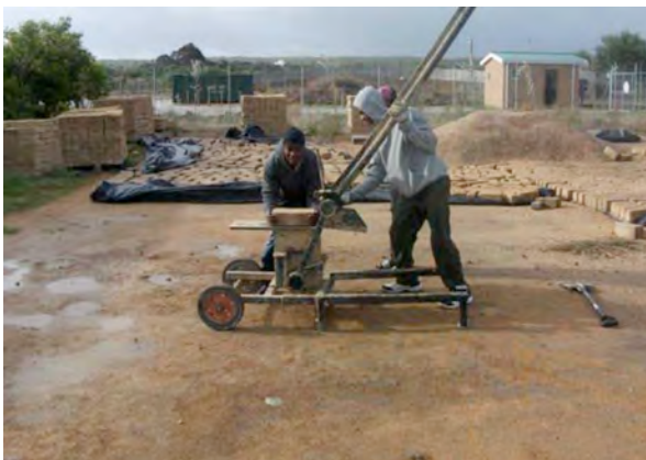
Fig_2.2. 17 & Fig_2.2. 18 : A sustainable hand-made building material, hand made on site using local sand and 5% cement/concrete stabiliser : Job creation, low carbon footprint, fire resistant, and creates a recyclable building material with no pollution.
