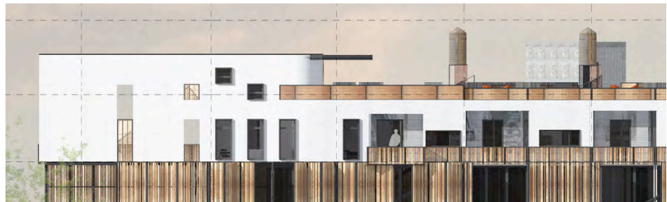
Fig_ii. 17 : View of the penthouse, showing the use of white brick, to coincide with the ground floor.
