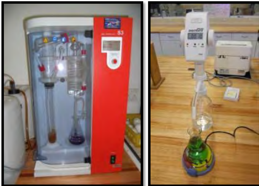
Figure 3.10: Distillation unit type S3 and sample during titration
