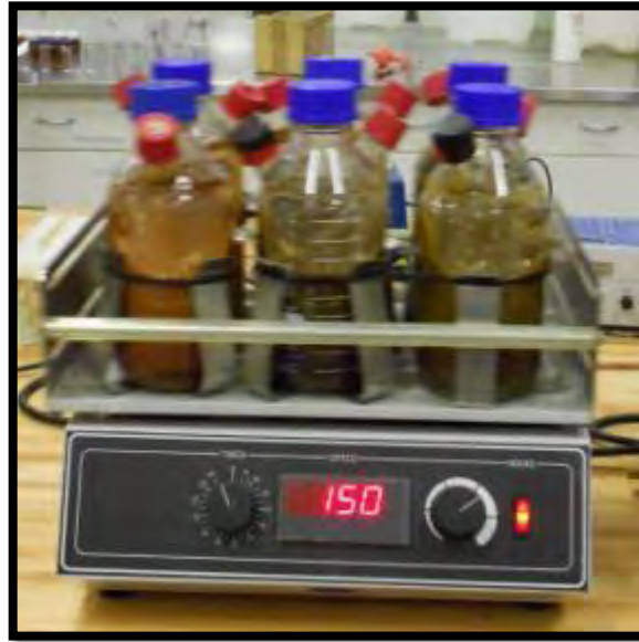
Figure 3.13: Batch test performed using CGR raw.
