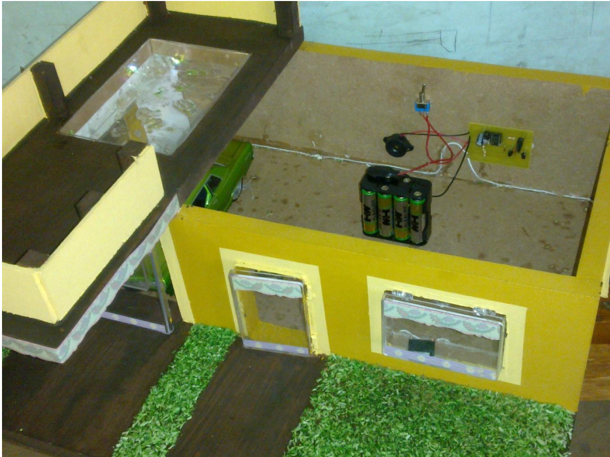
Figure 25: Installation of an alarm system in a model of a house
