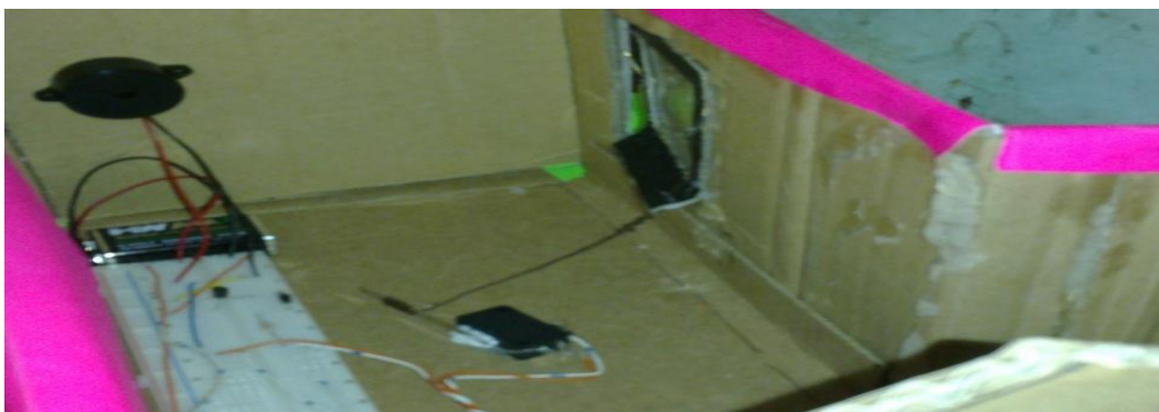
Figure 24: Use of a breadboard as an alternative to circuit board by group 11
