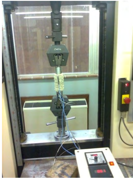
Figure 3-1: Instron5500R Setup for Steady State Tensile Temperature Tests
