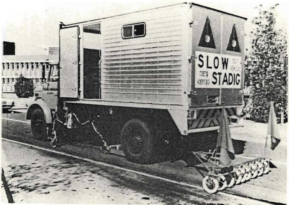
FIGURE A1.4 RUT DEPTH METER TOWED BEHIND LACROIX DEFLECTOGRAPH
