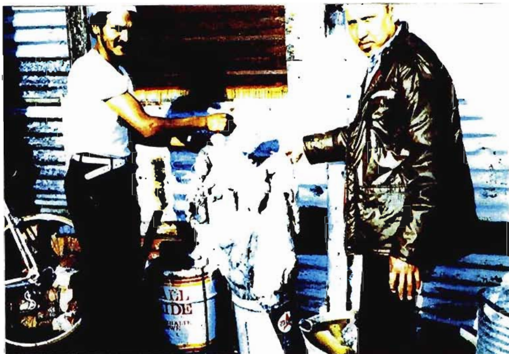
Plate XXXVI: The skin is taken out of the lime water.
