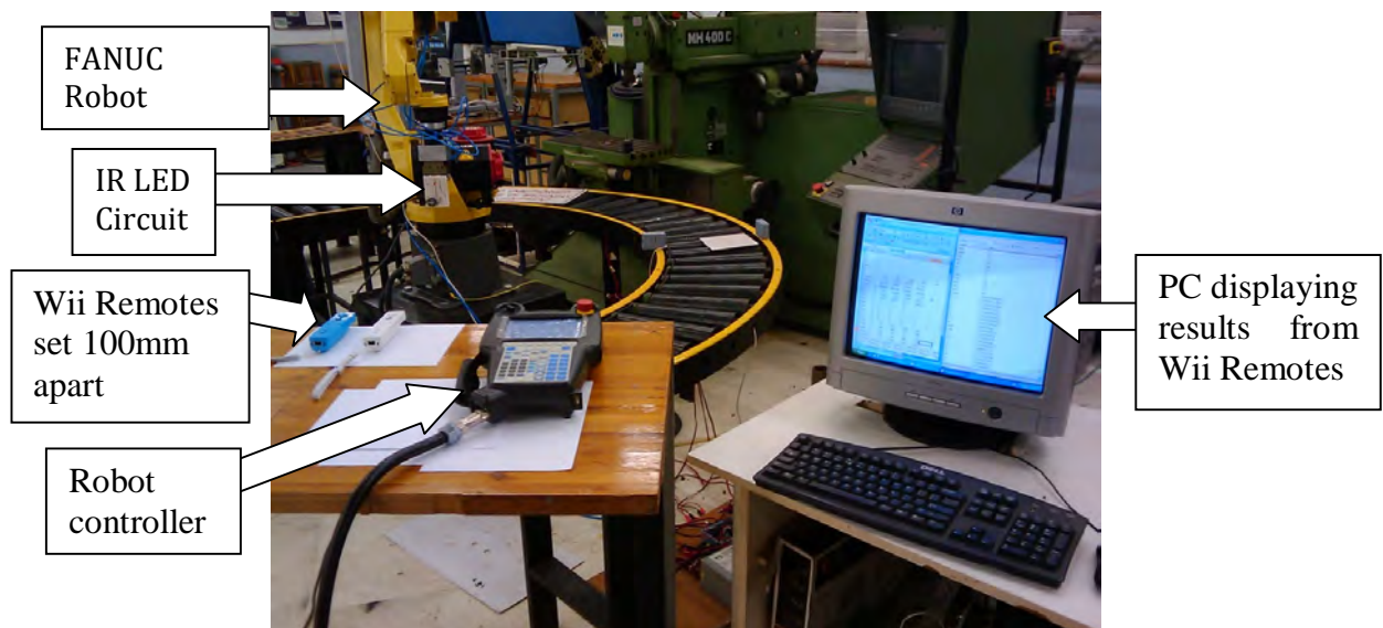
Figure 8-2: Positioning System Testing Setup
