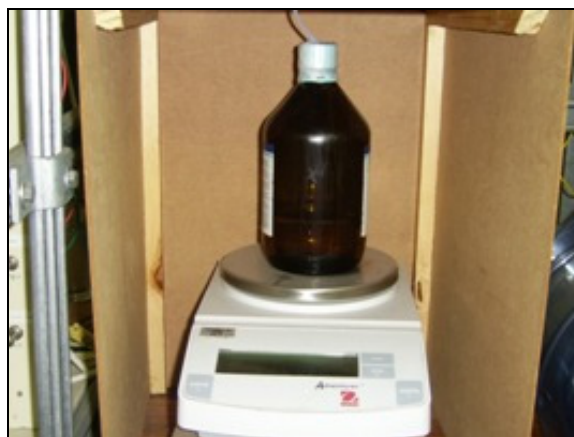
Fig D: Ohaus Adventurer TM balance used for determining mass of hexane feed.
