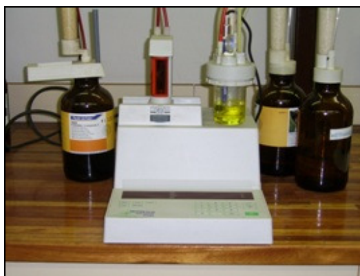
Fig A: Karl Fischer apparatus used for water determination.
