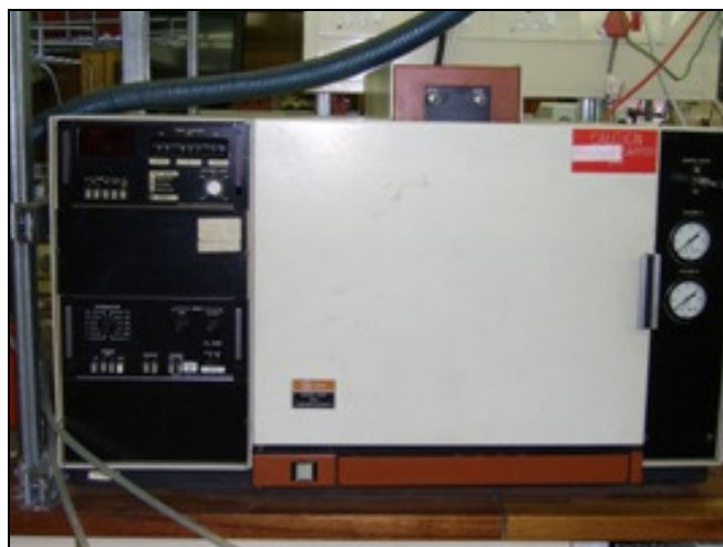
Fig F: Perkin Elmer Autosystem XL GC used for the quantification of hydrocarbons.
