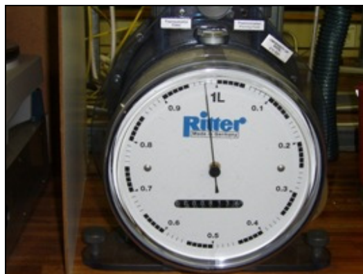
Fig C: Wet gas flow meter to measure total volume of gas.
