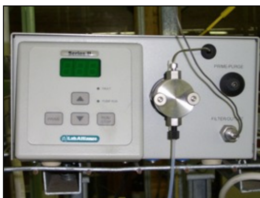
Fig. B: High performance liquid pump (HPLC) used for feeding n-hexane into the reactor.
