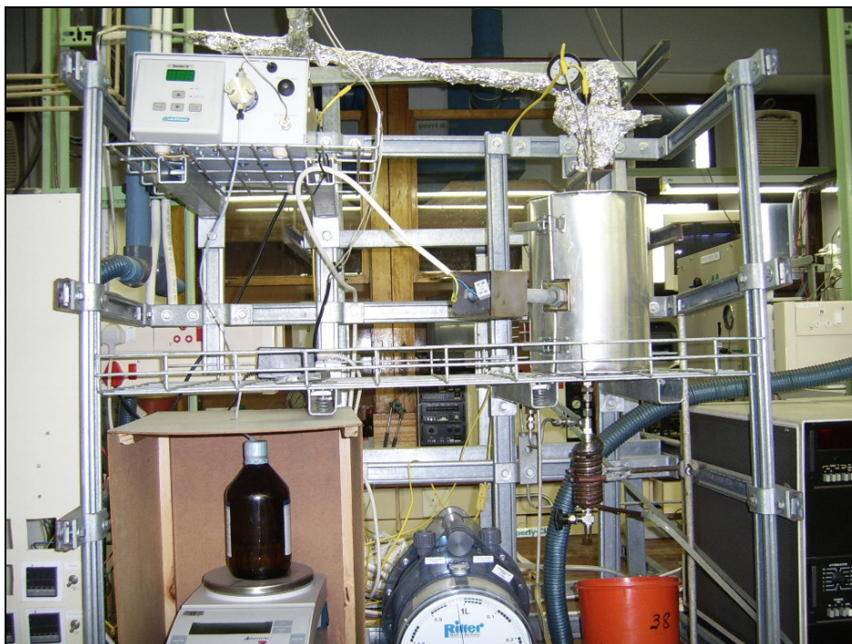
Fig I: Reactor set up used for testing n-hexane above the UFL.
