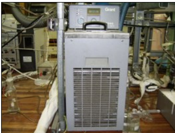
Fig E: A Grant LTD G -20 to 100°C chiller used for cooling products in catch pot.
