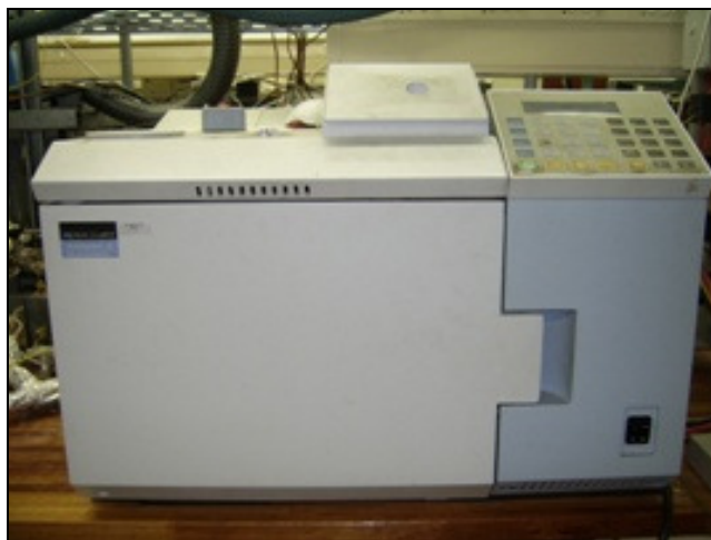
Fig G: Varian 3700 GC used for carbon oxide separation and quantification.
