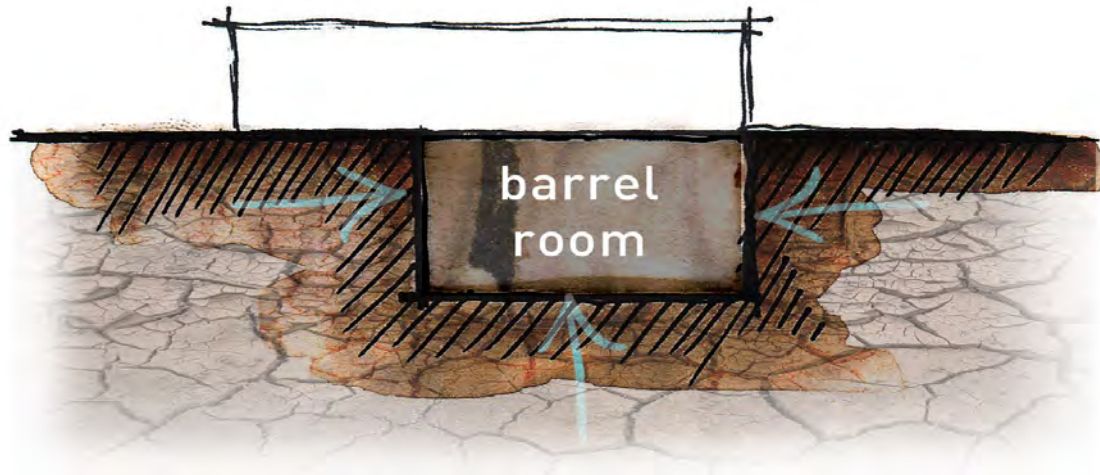
Spatial requirements for winemaking Figure 8.8 - Sketch showing natural cooling potential of winery caves.
