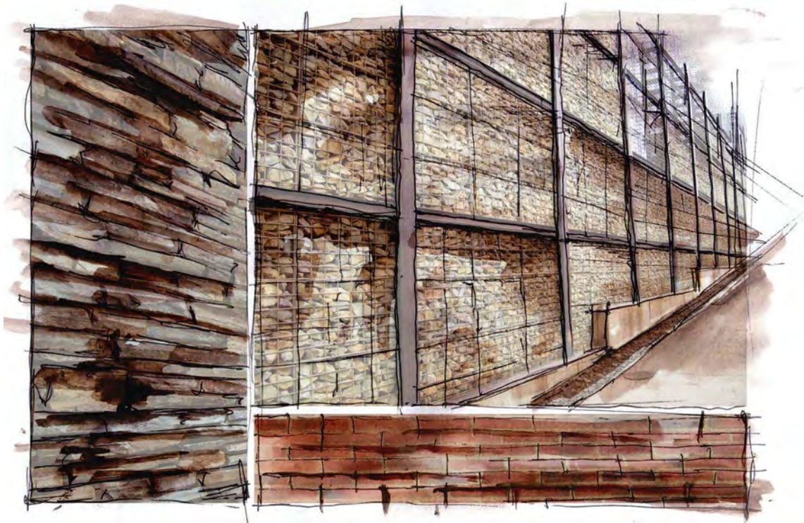
Apartheid Museum - Architectural collaboration Figure 5.25 (left) - dry-stack stone. Figure 5.26 (top right) - dry stack stone in galvanised metal cages held within a rusted steel frame. Figure 5.27 (bottom right) - non-standardised brickwork.
