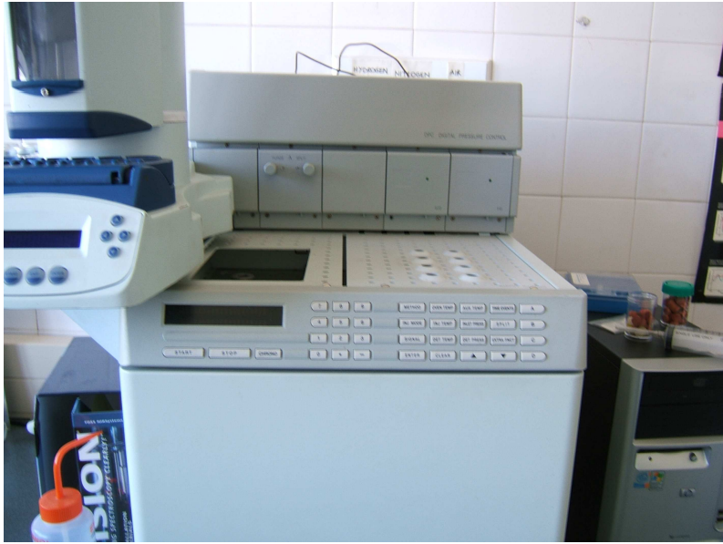
Figure A5: Gas chromatograph (GC) in conjunction with auto-sampler used in the measurement of ethylene gas evolution of Hass avocado fruit.
