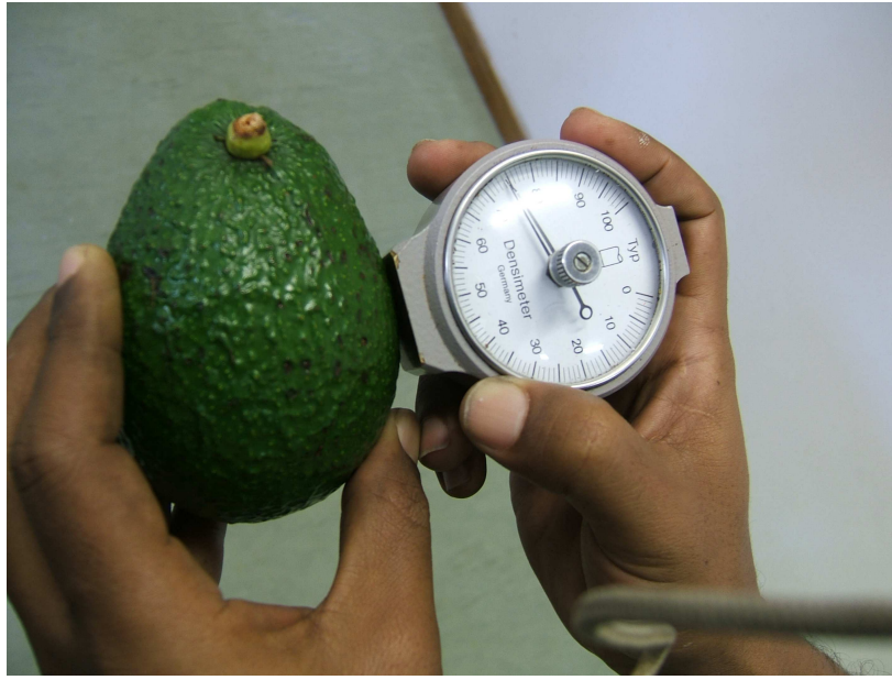
Figure A3: Hand-held firmness tester (Densimeter) being used to measure firmness of 'Hass' avocado fruit.
