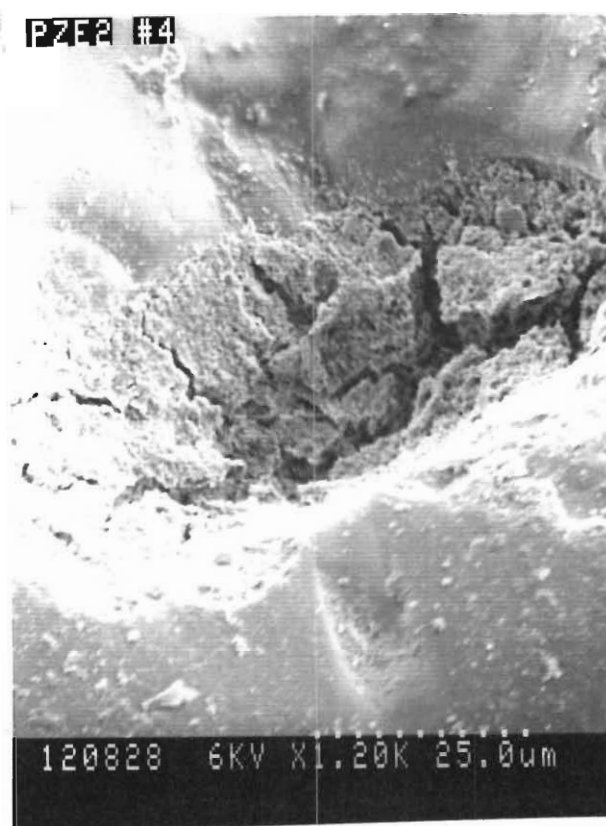
PLATE 4.05: SEM photomicrograph of a clay-filled open-mouthed pit in a zircon. Note the cracks in the surface coating over the clay-filling (SEM 120828).
