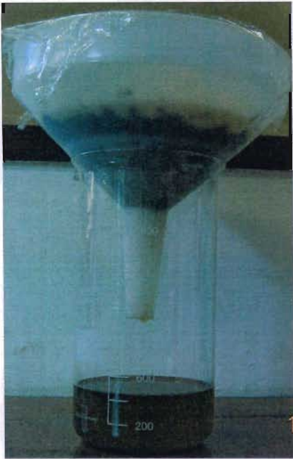
Plate 4-4: The Field Capacity Test Setup.
