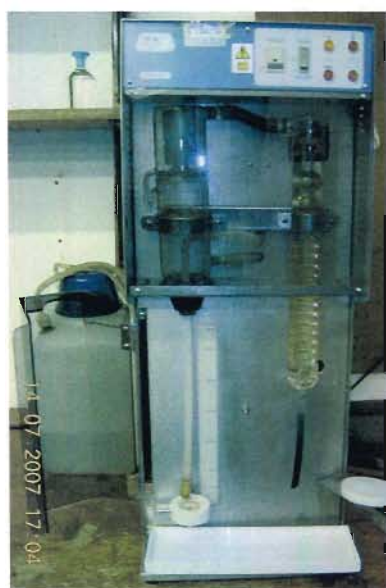
Plate 4-11: Nitrate and Ammonia Distiller. and Plate 4-12: Distillation Phase in Progress.
