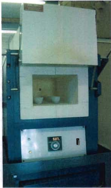
Plate 4-5: The Furnace used to Determine Volatile Solids.
