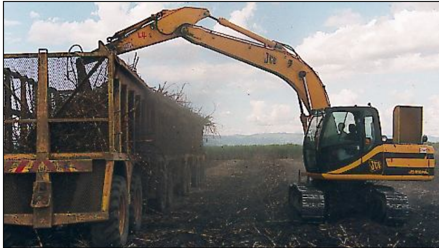
Figure 2.7 Excavator with a grab attachment loading sugarcane in-field
