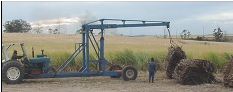
Figure 2.4 Bundled sugarcane being loaded by a mobile derrick crane at a transloading zone
