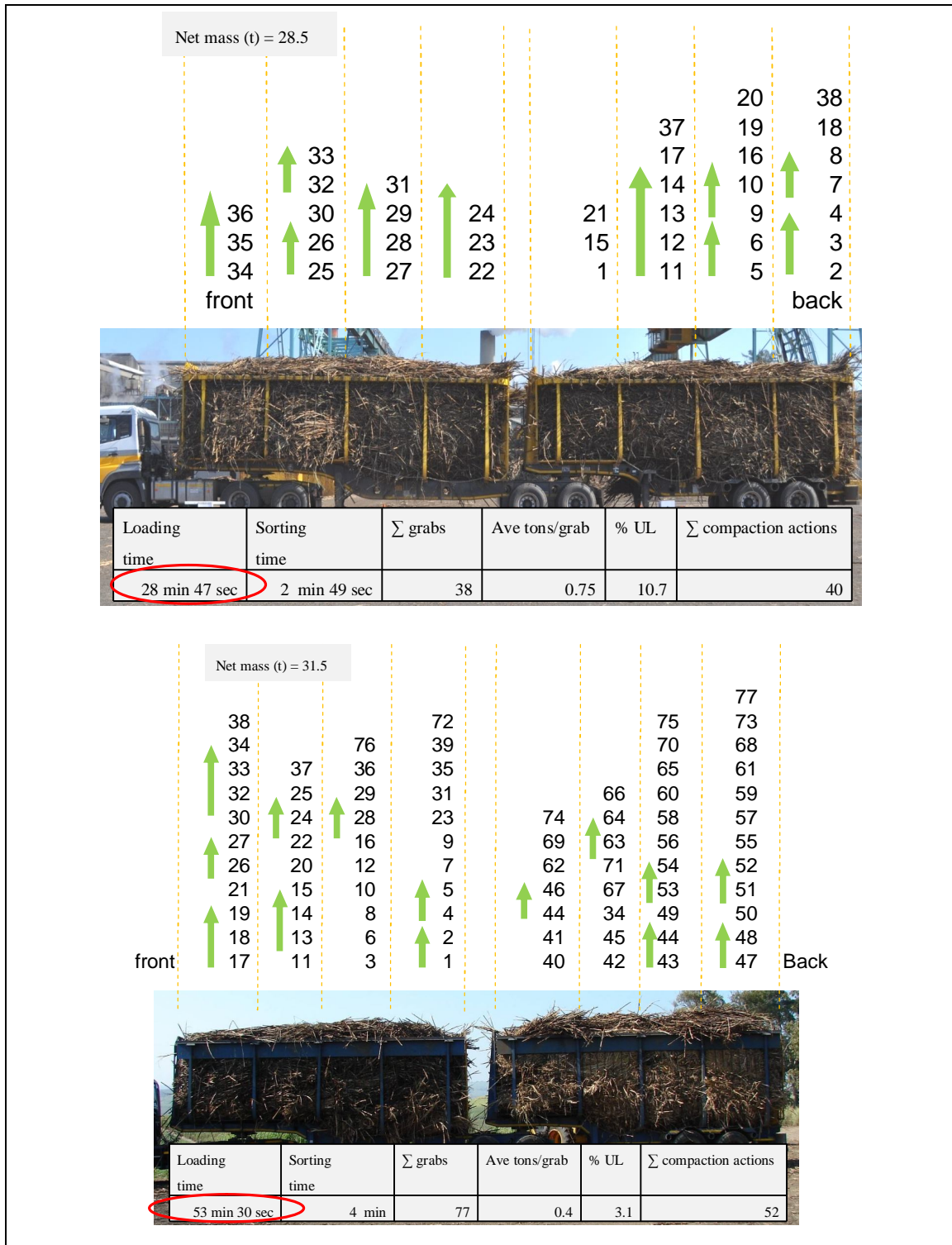
Figure 4.1 Images and sequence analyses for two loading operations assessed at transloading zones
