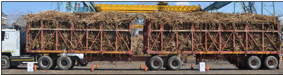
Figure 3.9 A consignment demonstrating the bread-loafing phenomenon
