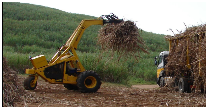
Figure 2.5 Three-wheel non-slewing grab-loader loading loose sugarcane at a transloading zone
