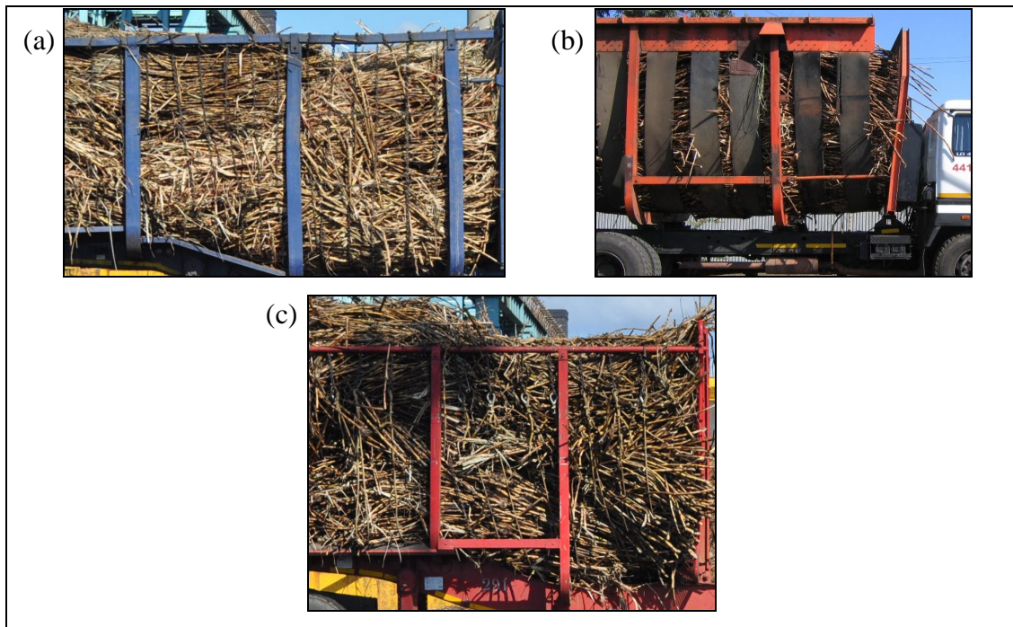
Figure 2.12 Various designs of trailers used to transport sugarcane, viz. (a) trailers with chains (b) trailers with belts in place of the chains and (c) trailers with ropes
