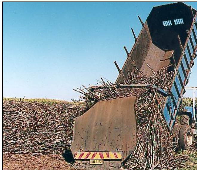
Figure 2.19 Rear-tipping trailer off-loading sugarcane at a transloading zone in South Africa
