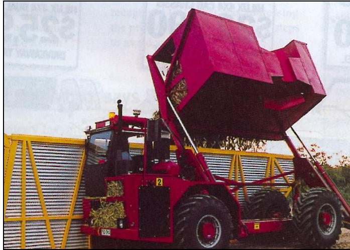
Figure 2.17 Sugarcane transloading by a hydraulic side-tipping trailer in Australia
