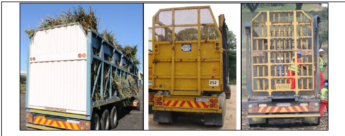
Figure 2.11 The different types of tailboards of sugarcane transport units in South Africa, closed, semi-closed and open (meshed)
