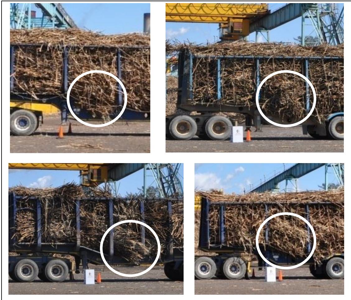
Figure 4.13 Demonstration of significant spillage at the unlevelled point of the trailer for interlink type vehicles.
