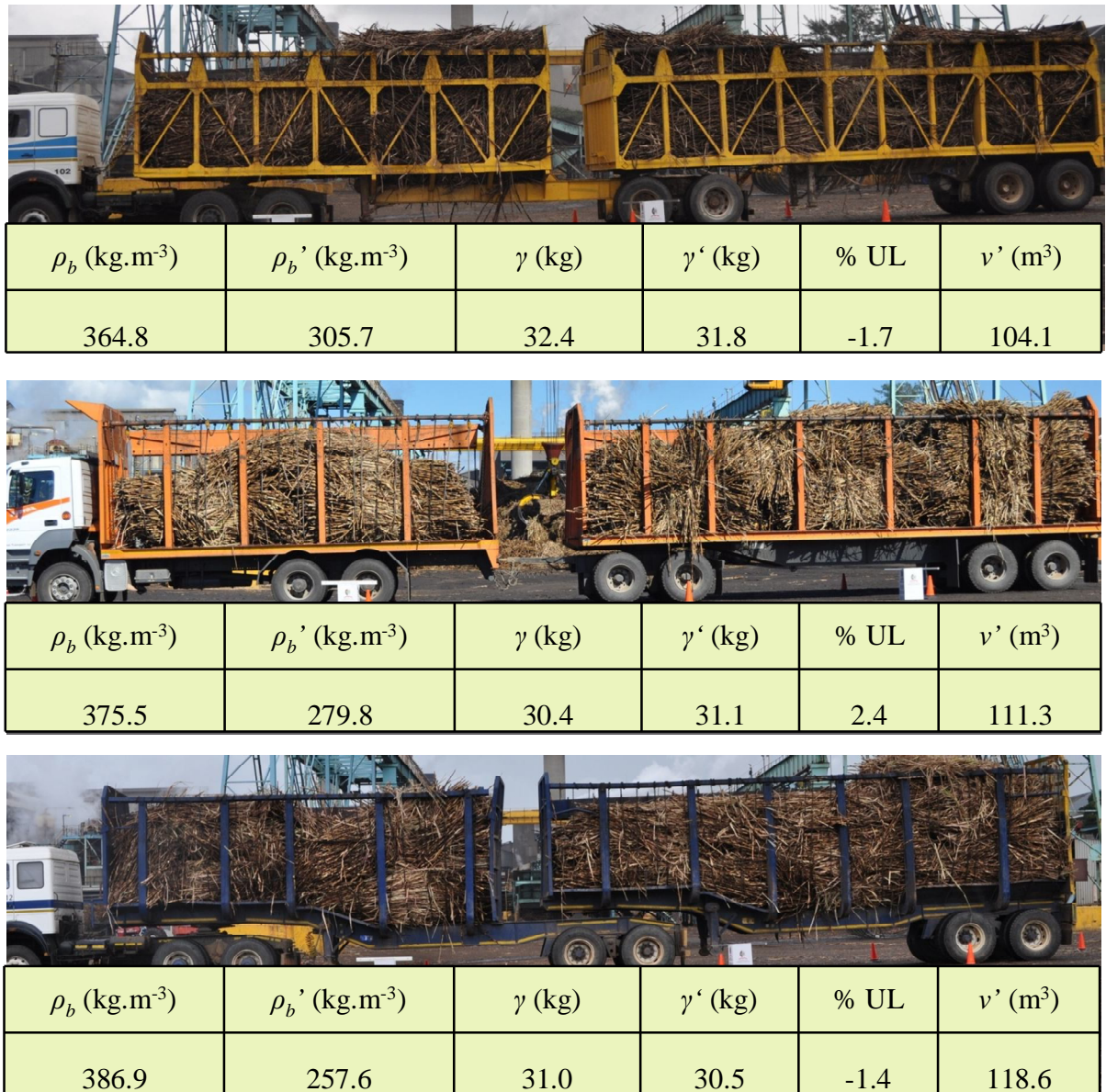
Figure 4.8 Typical consignments which arrived with the \rho_b > \rho_b'
