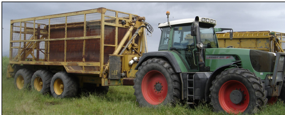
Figure 2.18 A South African transloading hydraulic side-tipping trailer
