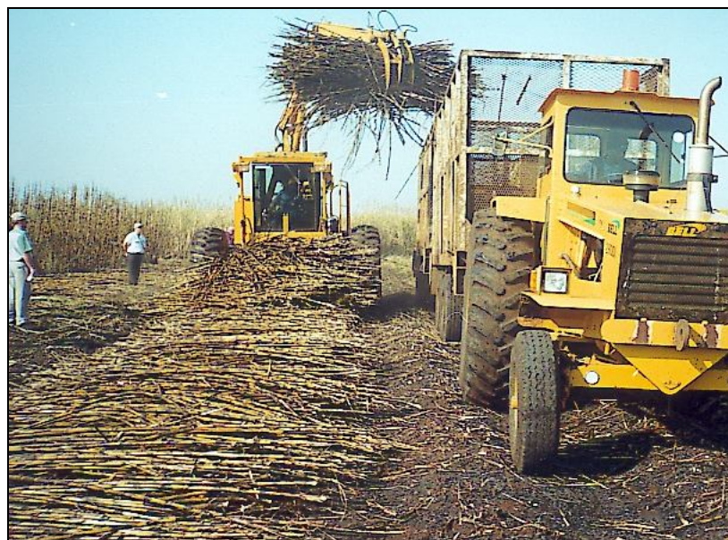
Figure 2.6 Push-pile slewing grab-loader loading loose windrowed sugarcane in-field
