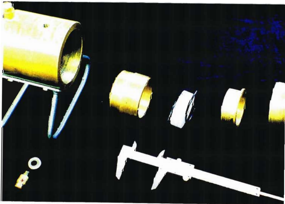
Plate 4.2 Photograph showing the different parts of the Ohle cell. (Vernier calliper open at 50 mm).
