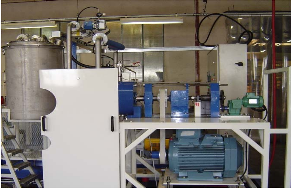
Figure 3.1: Pilot refiner fitted with pulper, water heater, sampling carousel and electronic cabinet
