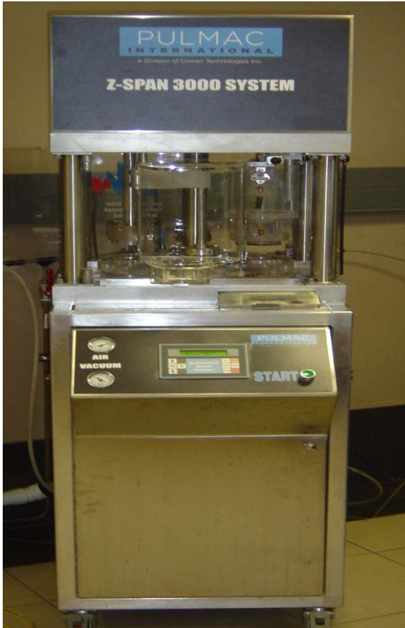
Figure 3.7: Pulmac automatic sheet former (left) and the wet zero span tester used to measure the fibre strength and bonding index of fibres
