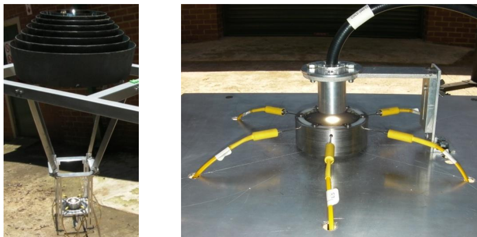
Figure 9.2 (left) Calorimeter positioned at concentrator focal point to characterise the performance of the composite material RAC and (right) fibre optic cable directed onto the calorimeter to determine exit flux concentration.
