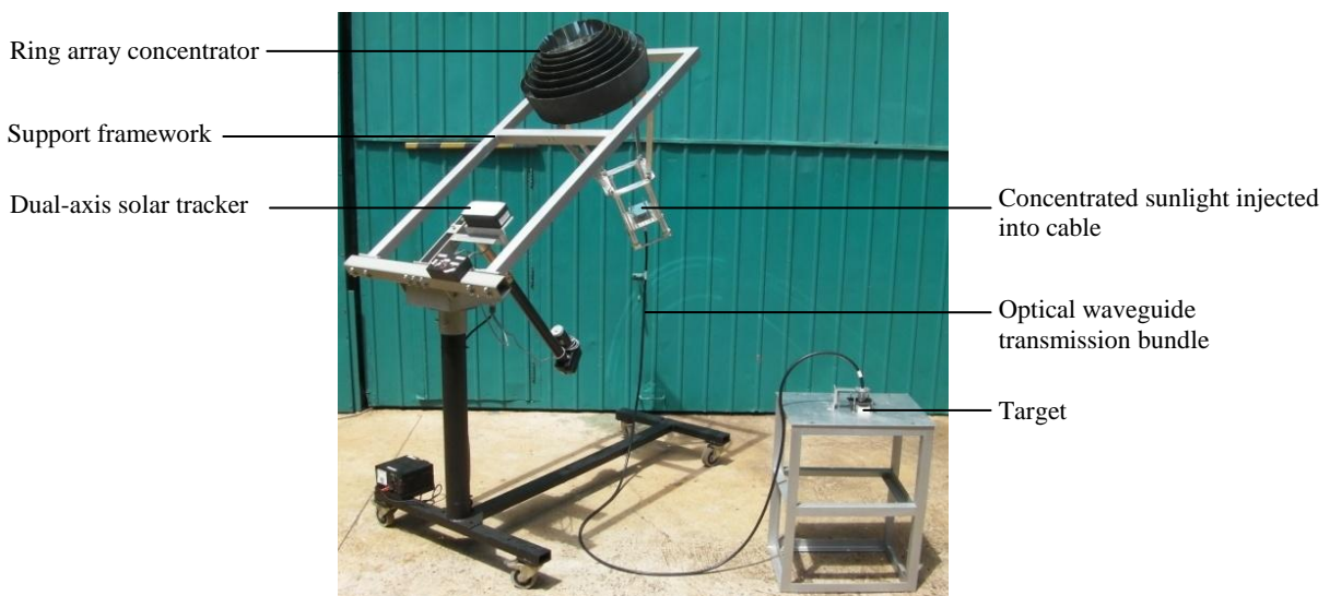
Figure 3.1 FOCUS consisting of a ring array concentrator integrated with an optical waveguide bundle to provide high-flux levels remote from the collector.
