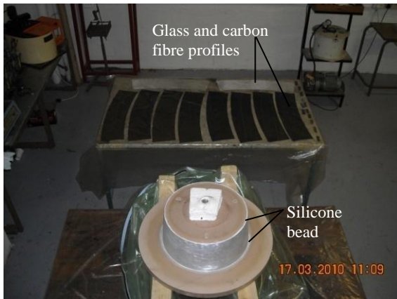
Figure 5.3 (left) Aluminium profile after bonding with a bead of silicone to prevent resin offset between the metal surface and mould. Glass and carbon fibre profiles were hand impregnated with resin for the wet lay-up and second vacuum bagging process. (right) Second vacuum bag process with peel ply, perforated film and bleeder surrounding the lay-up to improve the composite finish.
