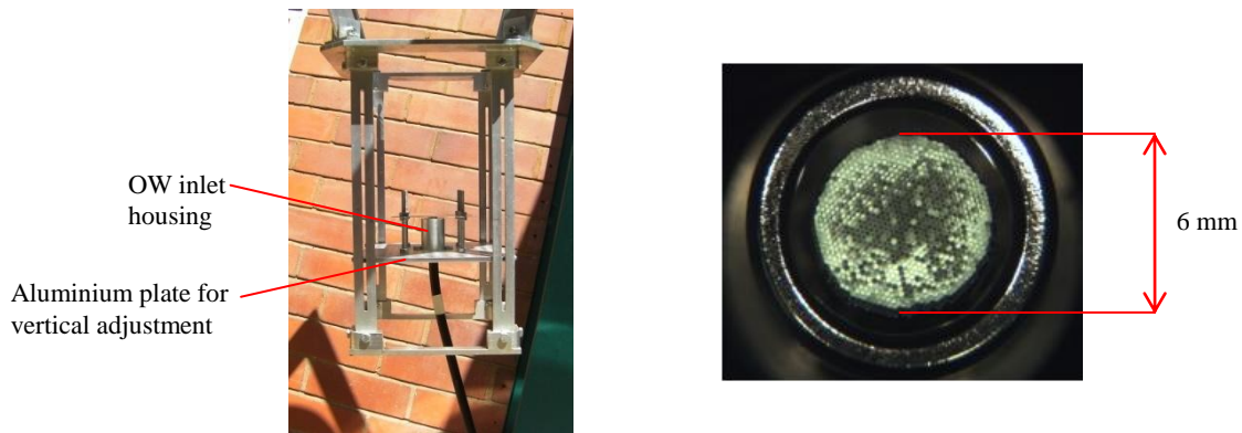
Figure 3.4 (left) Housing of the inlet to the fibre optic cable. The aluminium structure allows vertical adjustment of the focal point. (right) Representation of the inlet and outlet 6 mm diameter fused ends of the fibre optic waveguide.
