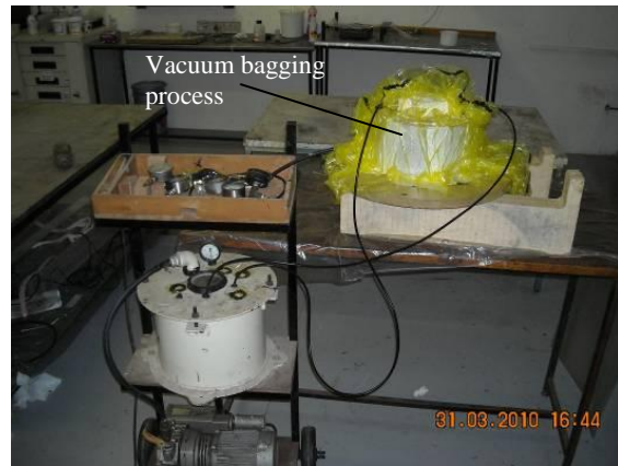
Figure 5.3 (left) Aluminium profile after bonding with a bead of silicone to prevent resin offset between the metal surface and mould. Glass and carbon fibre profiles were hand impregnated with resin for the wet lay-up and second vacuum bagging process. (right) Second vacuum bag process with peel ply, perforated film and bleeder surrounding the lay-up to improve the composite finish.
