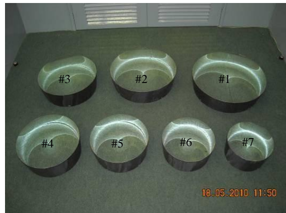
Figure 5.4 (left) After curing vacuum is removed and the element is demoulded using tabs. (right) The completed seven FRP elements #1 to #7, anticlockwise from back right.
