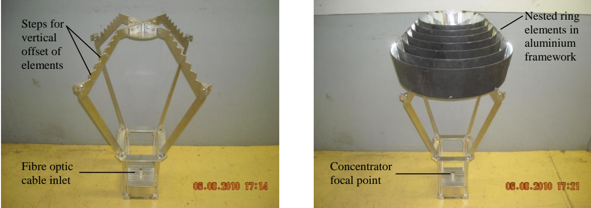
Figure 5.6 Machined aluminium framework to house reflective elements and fibre optic cable (left). Fibre reinforced plastic reflective elements nested in support framework (right).
