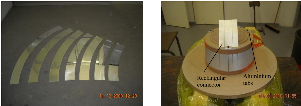
Figure 5.2 (left) Developed conic profiles of Miro 4 polished aluminium for the elements. (right) Profile for element #7 strapped to the tooling board mould before first lay-up. A vacuum is applied during bonding of the aluminium over the mould to enforce the paraboloidal shape.
