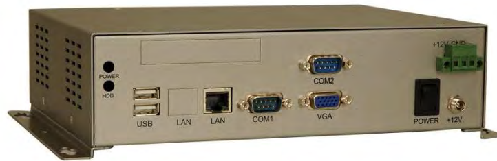
Figure 5.4: Single board computer in enclosure
