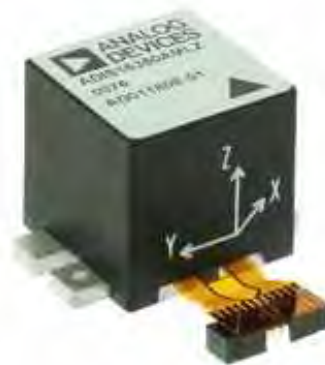
Figure 4.6: Analogue devices: ADIS16350 combined accelerometers and gyroscopes
