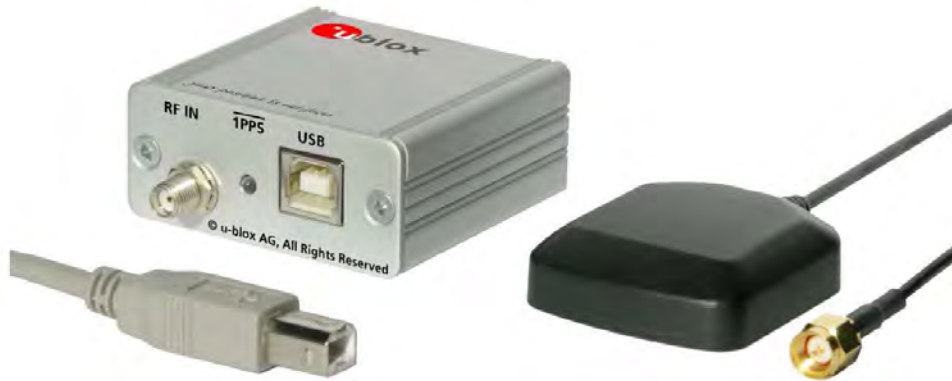
Figure 4.17: u-blox EVK-5H GPS evaluation kit
