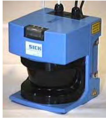
Figure 4.13: SICK LMS200 laser range finder
