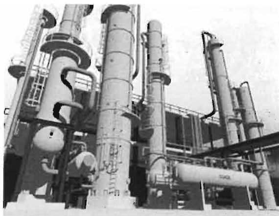
Figure 1-1 : Typical Cylindrical Pressure Vessels
