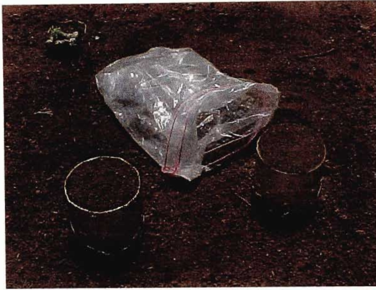
Fig. 4.6 Two plastic soil microlysimeters of low thermal conductivity, before insertion into the soil. Aluminium foil with high thermal conductivity is covered at the bottom of the cylinders. In the background is a zip lock bag where the microlysimeters are inserted and then folded in order not to protrude above the soil surface
