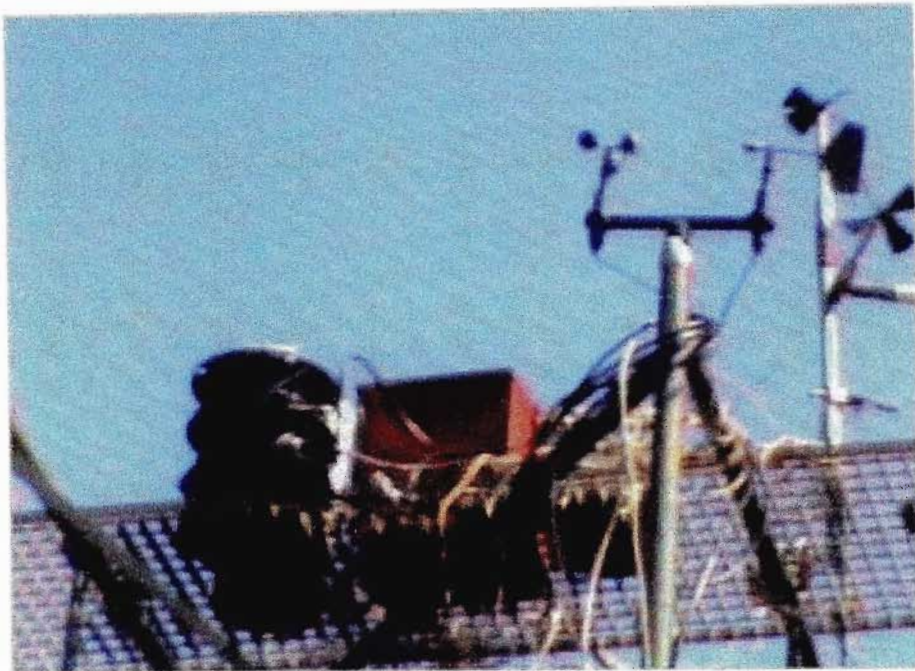
Fig. 4.4 Equipment supported by scaffolding , the red oxide metal box housed the datalogger and batteries, on the right background is the 3D propeller anemometer and the right foreground is the RM young anemometer
