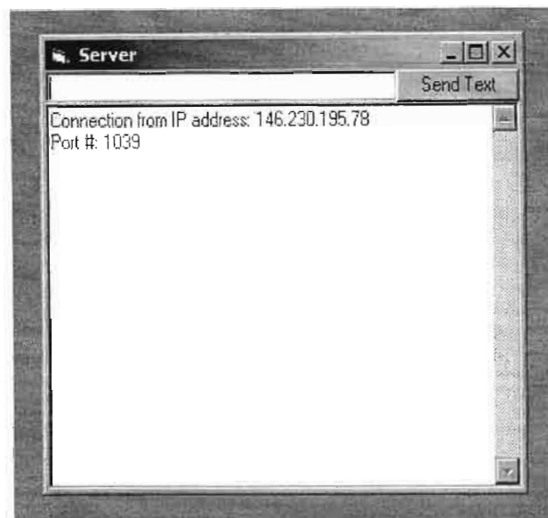
Figure 9.8. The Server.frm form. Note the server has connected to IP address 146.230.195.78, which is the Camera Selector Client.
