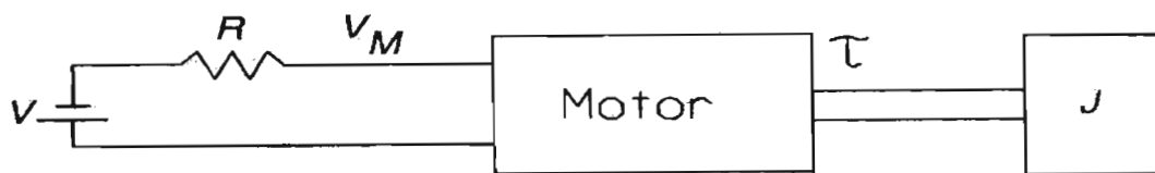
Figure 3.2. The “black-box” motor with drive and load.
