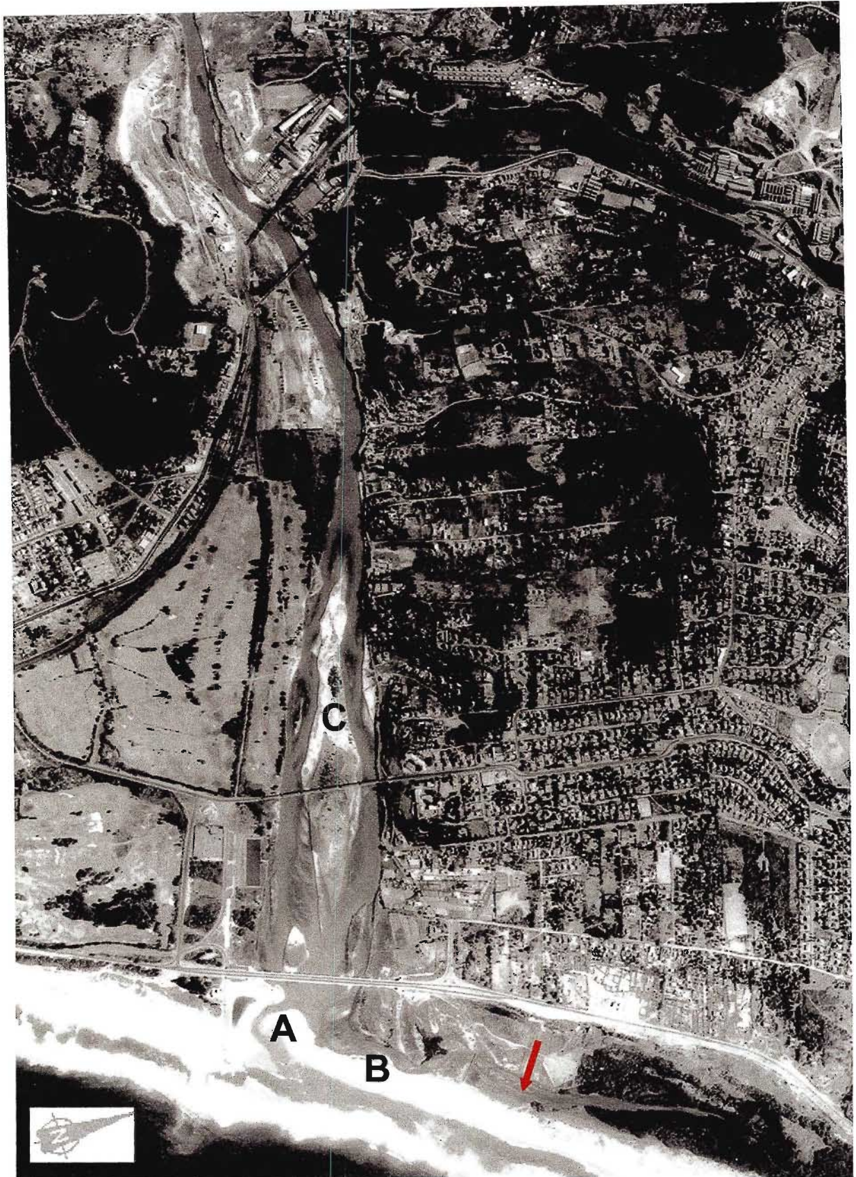
Aerial Photograph 4.2: The Mgeni River Estuary in 1959 (A, B & C). Note the reduction of the channel in the Beachwood Mangroves and the formation of the midstream island.
