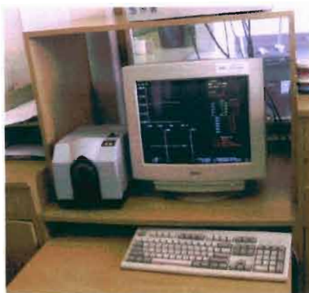
Figure 4-6: The Spectrophotometer set-up
