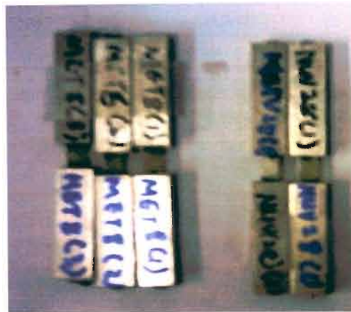
Figure 3-6: Specimens ready for compression test
