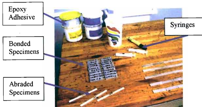
Figure 3-3: Gluing of tabs onto Specimens
