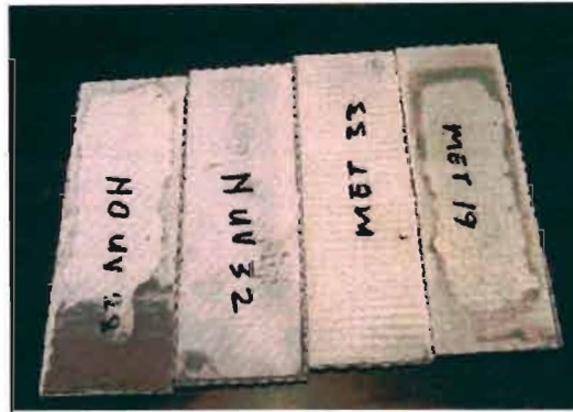
Figure 5-19: The colour change on water immersed laminates
