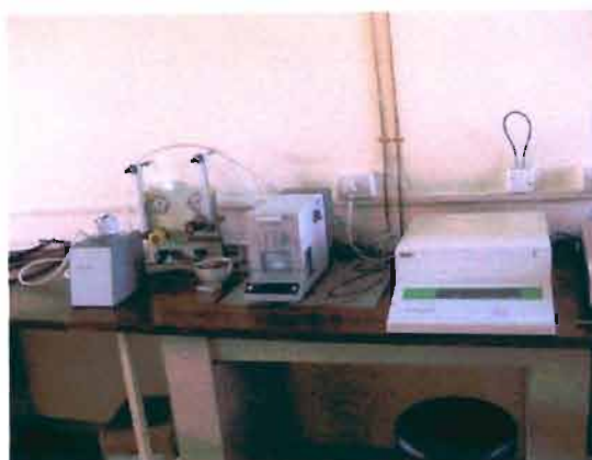
Figure 4-7: The Differential Scanning Calorimeter set-up
