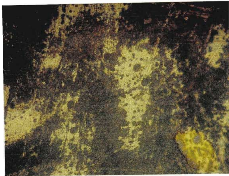
Figure 6.14: Microstructure in neck region of tensile fracture of alloy 304. (Mag. 400x)
