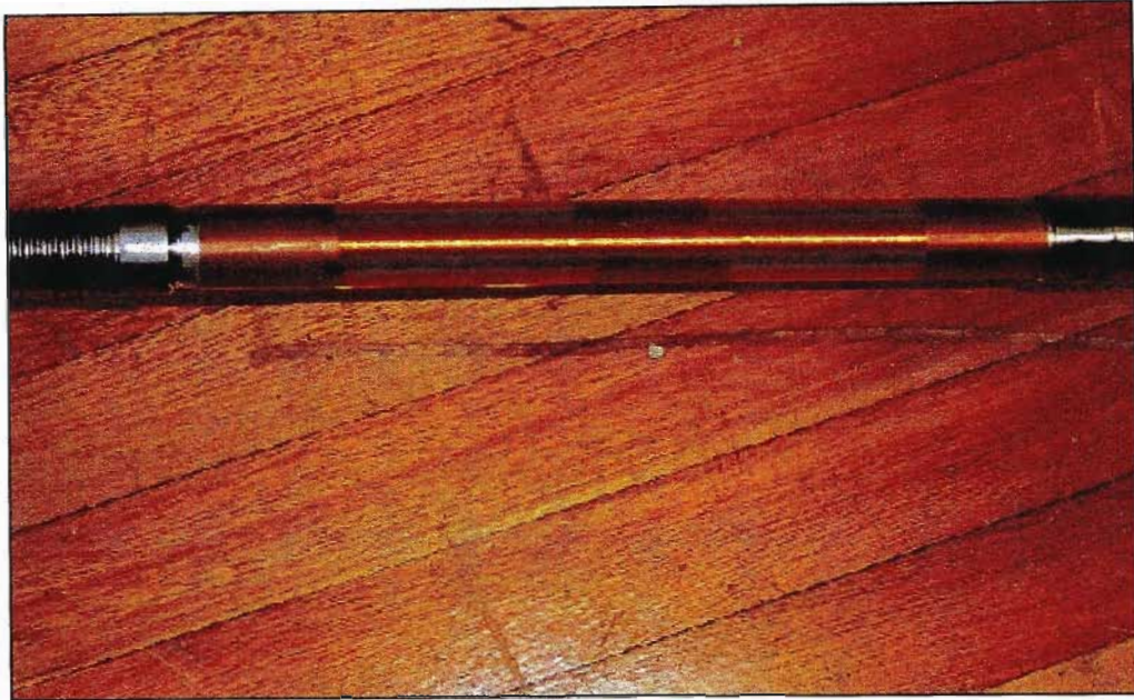
Figure 6.7: A coil was wound around the necked down section of the tensile sample
