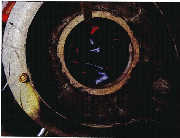
Figure 6. 2: Remelted iron can be seen on the top of the charge, which is beginning to melt.
