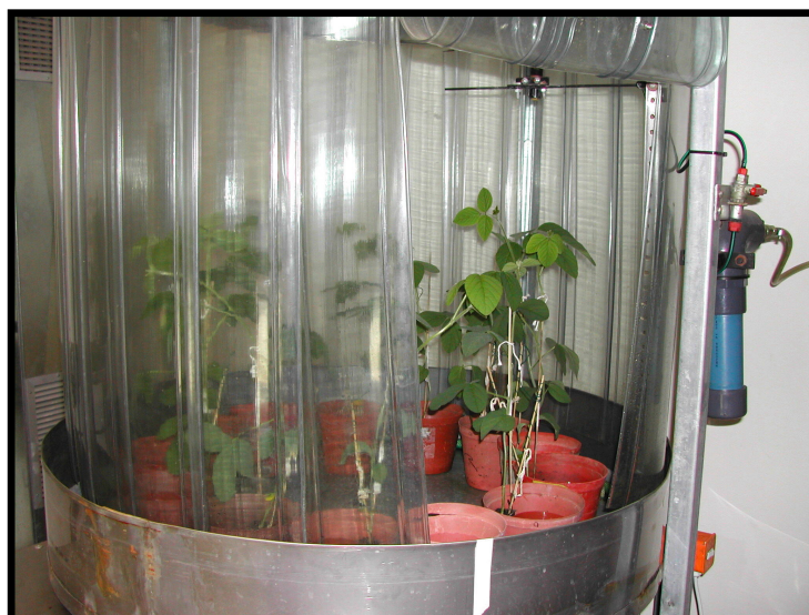
Figure 5.2 Herbicide sprayer used to apply fungicides to soybean plants.
