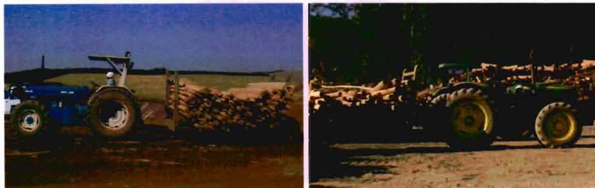
Figure 5.3 Agricultural tractor trailer combinations used for the extended primary transport phase in the two study areas. (Study Area A) Ford 8030 with 5 ton bundle trailer (left) (Study Area B) John Deere 6320 with 5 ton bundle trailer (right)
