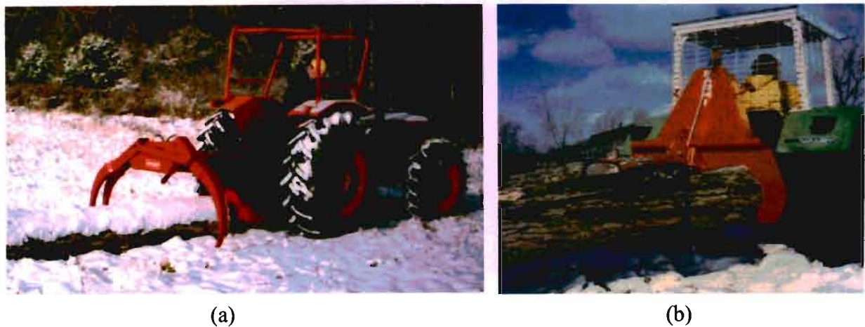
Figure 2.10 Skidding attachments for agricultural tractors (a) grapple (b) winch
