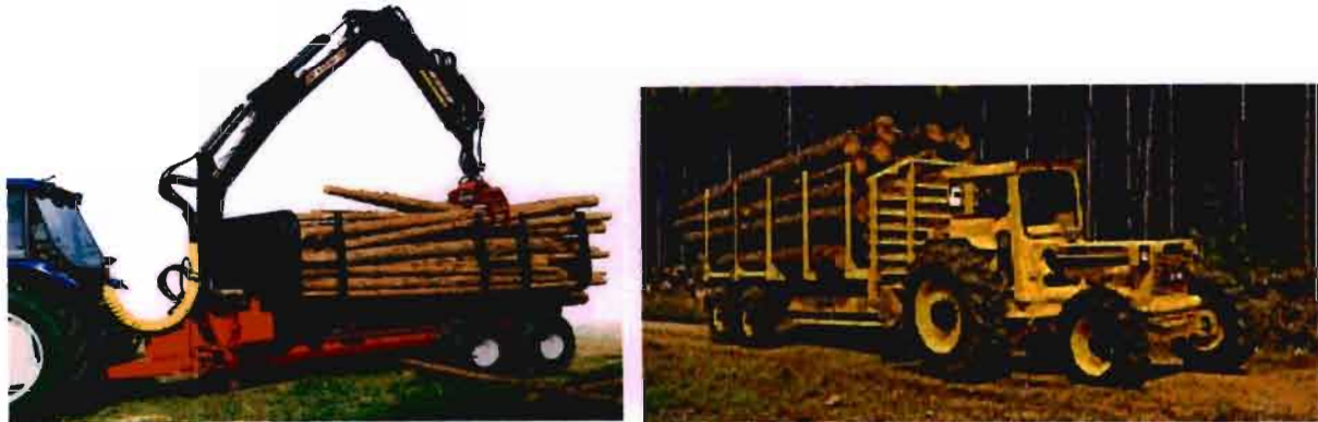
Figure 2.12 Tractor trailer combinations used for forwarding (a) Agricultural tractor with bogie axle trailer and knuckle boom loader (b) Haulage tractor and trailer
