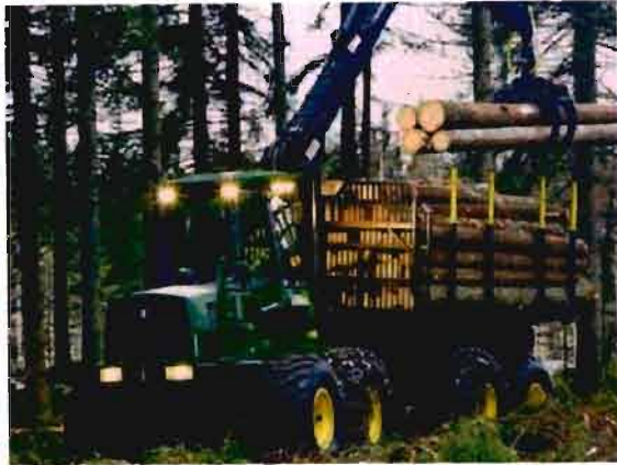
Figure 2.11 An eight and six wheel drive forwarder each with a mounted knuckle boom crane for self loading and off loading
