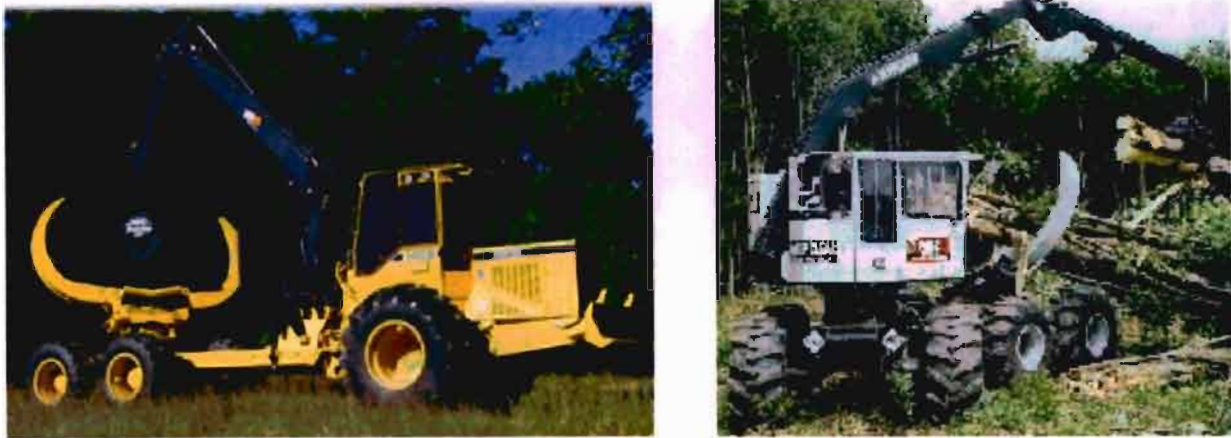
Figure 2.9 Clambunk skidders showing the inverted grapple and the knuckle boom crane
