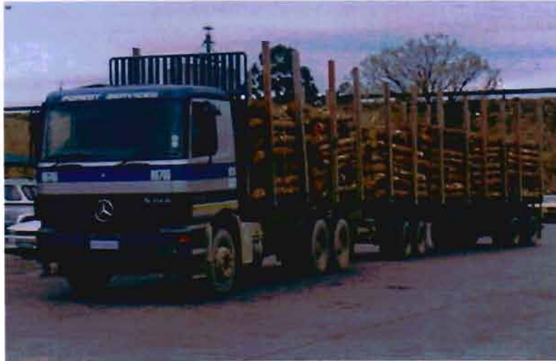
Figure 5.5 Rigid type truck with drawbar trailer used for secondary terminal transport in the two study areas
