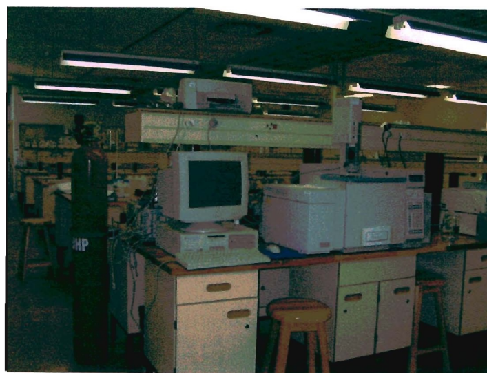
Figure 2.43: The Hewlett Packard 6890 gas chromatography instrument coupled to a Hewlett Packard 6890 mass-selective detector.
